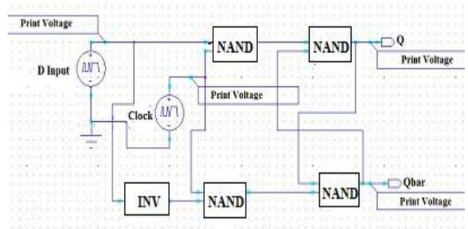
Figure 6: Schematic of D Latch using Clock
