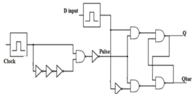
Figure 8: D Latch using Pulsed Clock
