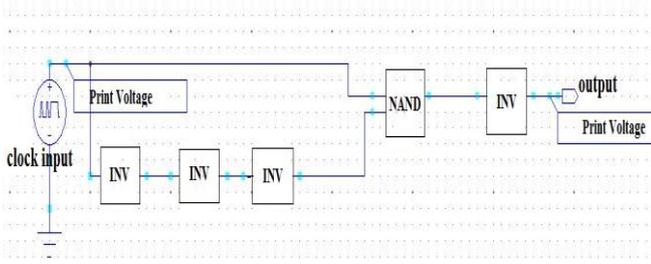
Figure 3: Schematic of pulse generator
