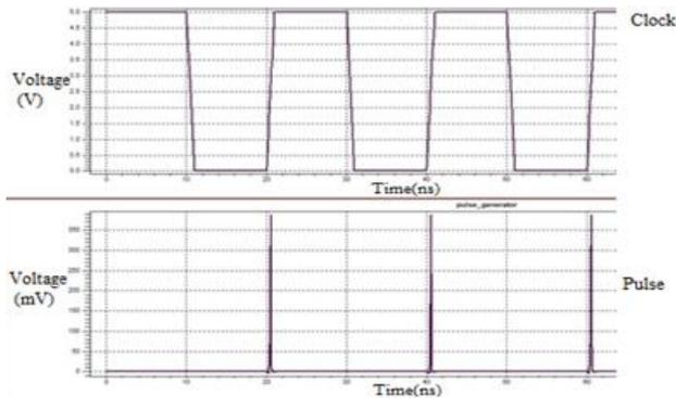
Figure 4: Pulse generator waveform
