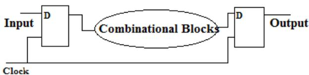
**Figure 1:** Basic sequential circuit
