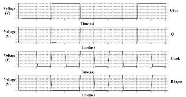
Figure 7: D Latch waveform
