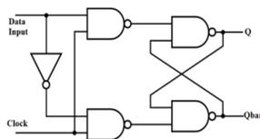
Figure 5: D-Latch using NAND
