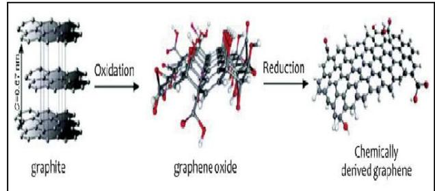
Fig. 4. Conversion process of graphite into graphene [22]
