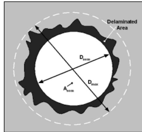
Fig. 6. Delamination [24]
