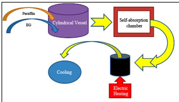
Fig. 3. Preparation of expanded graphite [20]
