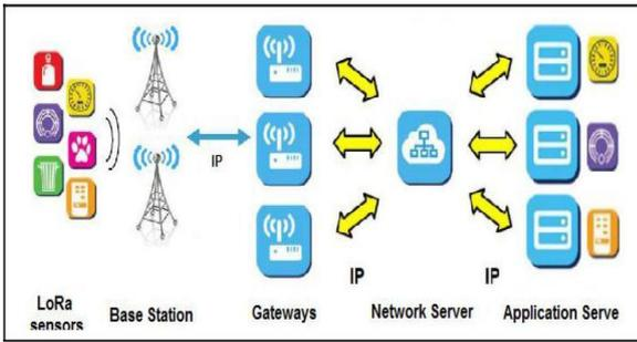
**Figure 1:** LoRaWAN network architecture
