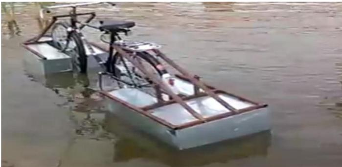
**Fig 5 : Floating bicycle during floatation test**
