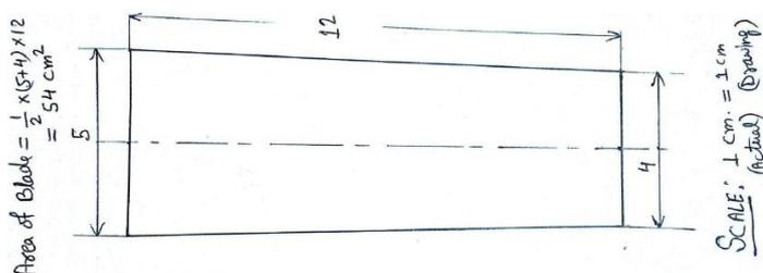
**Fig 4: Shape of the blade**
