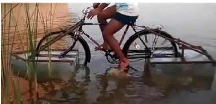
**Fig 7: Driving test inside the water**
