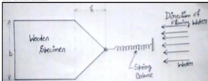
Fig 3: Schematic diagram of setup for the testing of shape of float
