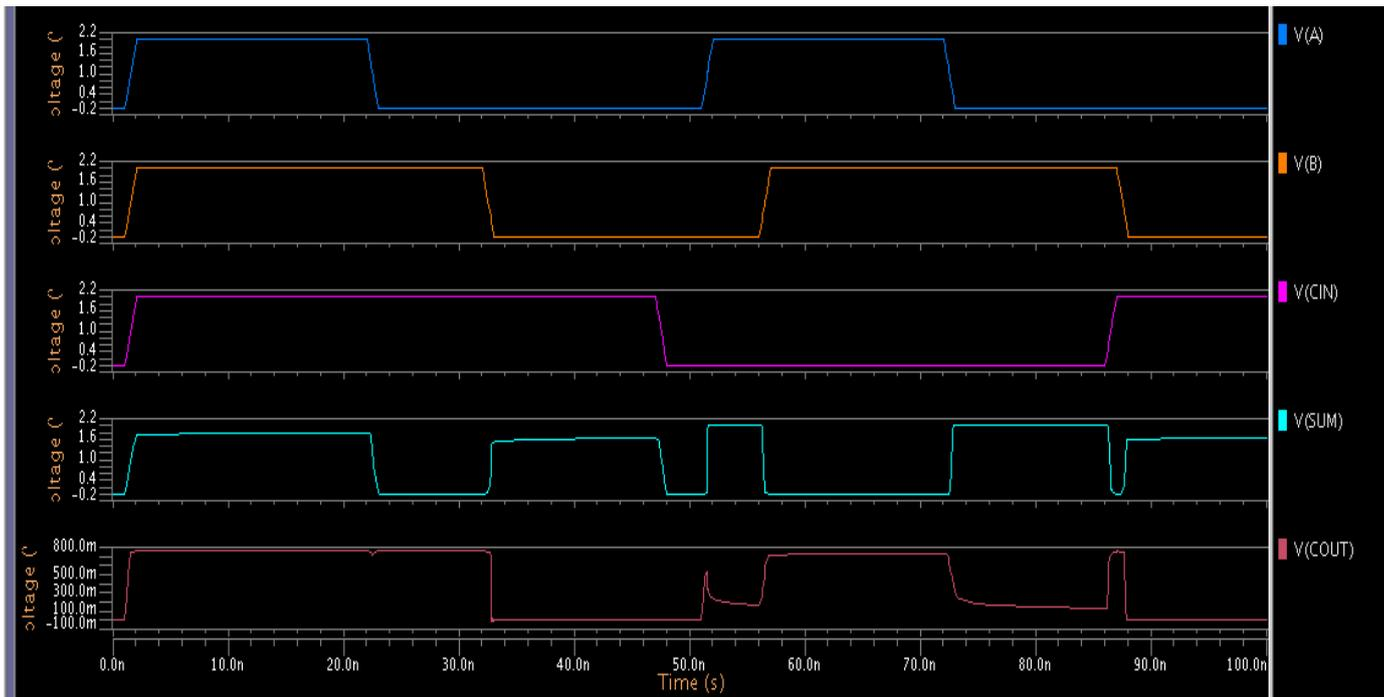
**Fig (7).** Waveform of a one-bit GDI FA circuit
