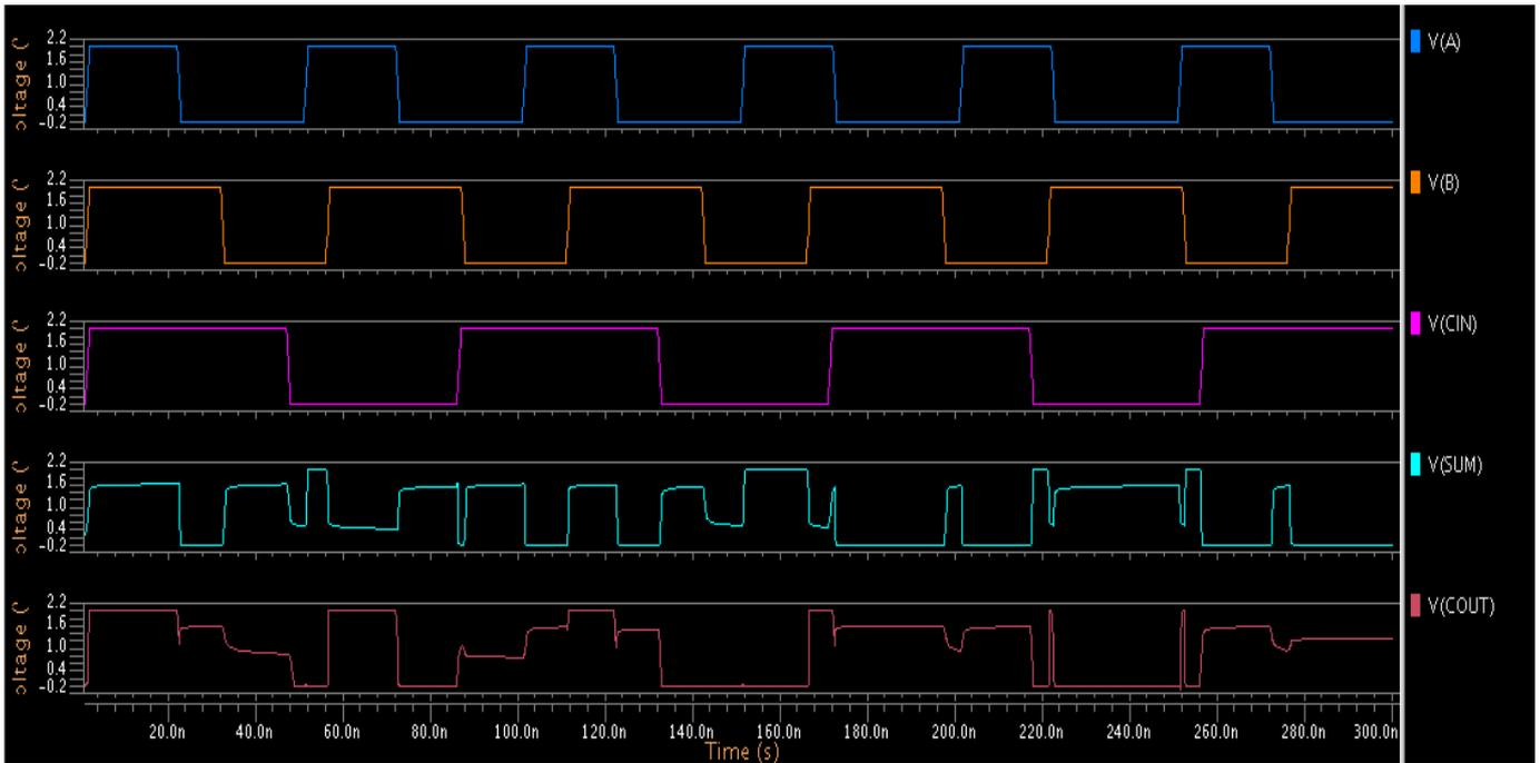
**Fig (6).** Waveform of a one-bit SERF FA circuit
