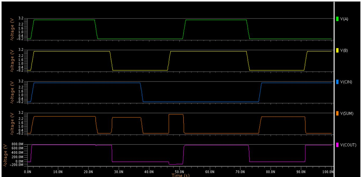
Fig (8). Waveform of a one-bit Mod-GDI FA circuit
