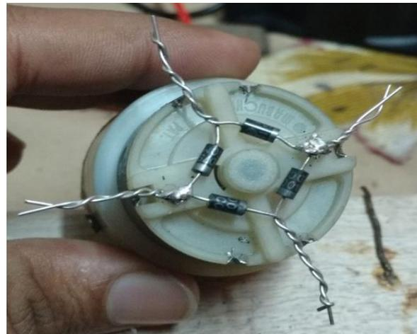
Figure 3: Diode Bridge
