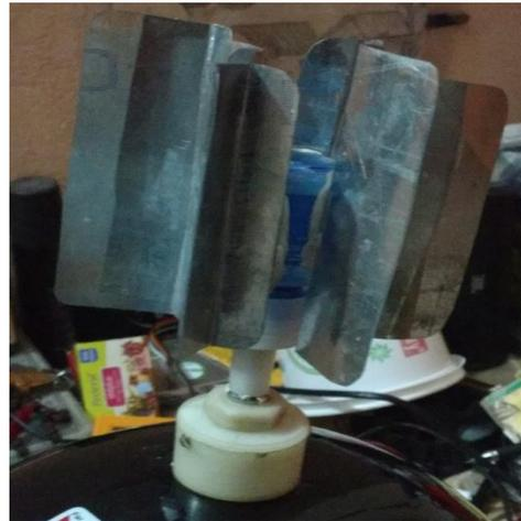
Figure 2: DC motor and blade assembly
