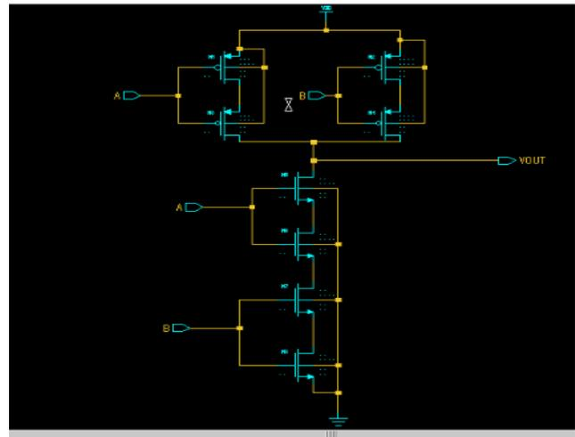
Fig. 5. Stack NAND circuit
