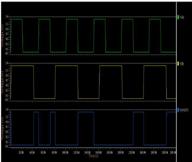
Fig. 12. Input-Output waveforms of NOR circuit using stack technique
