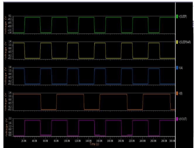
Fig. 15. Input-Output waveforms of NOR circuit using MTCMOS plus Stack technique
