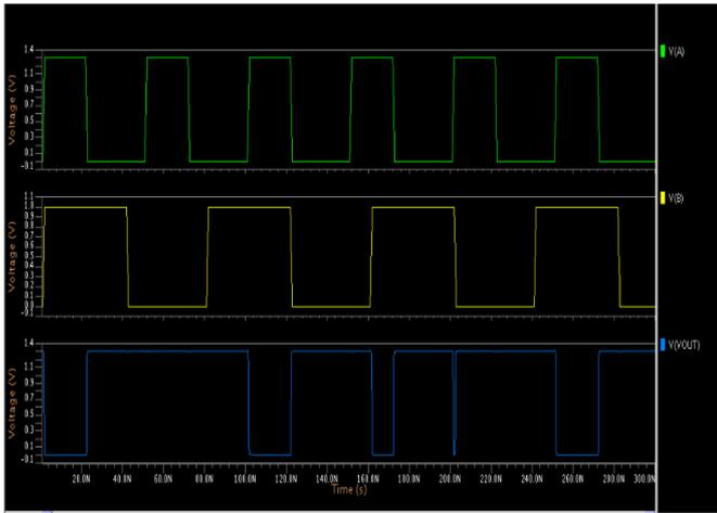
Fig. 11. Input-Output waveforms of NAND circuit using stack technique
