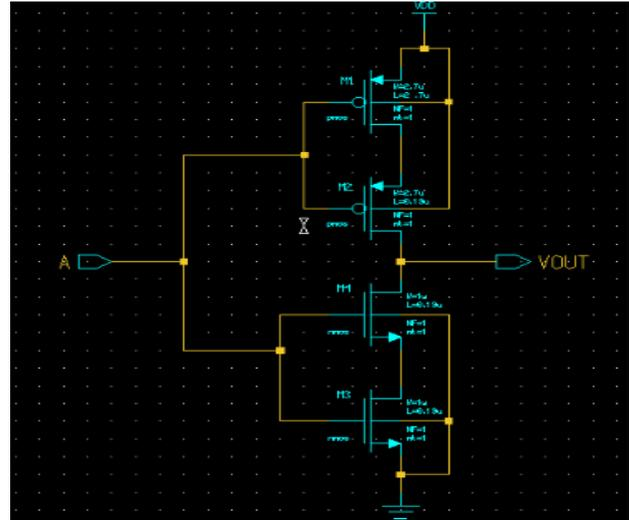
Fig. 4. Stack Inverter circuit
