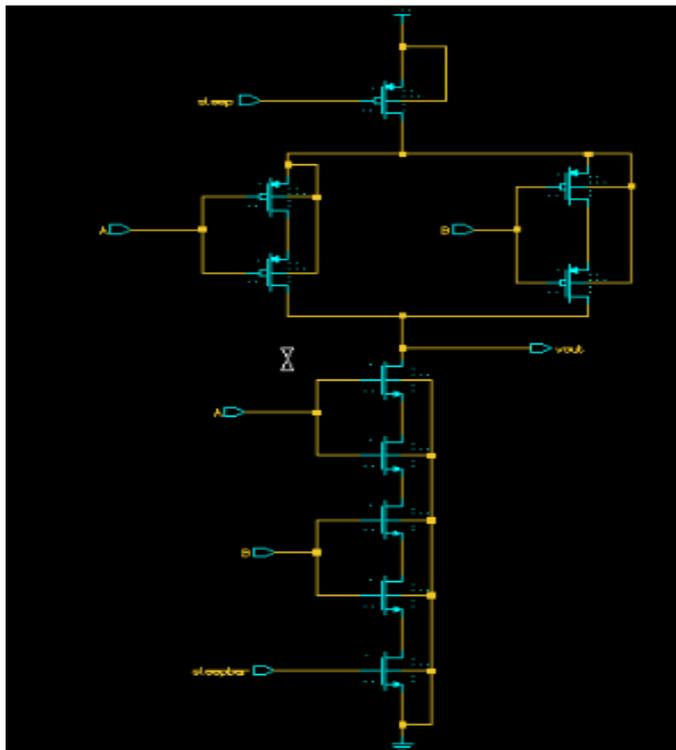
Fig. 8. NAND circuit using MTCMOS plus Stack technique
