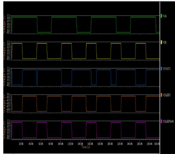
Fig. 14. Input-Output waveforms of NAND circuit using MTCMOS plus Stack technique
