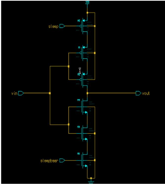
Fig. 7. Inverter circuit using MTCMOS plus Stack technique
