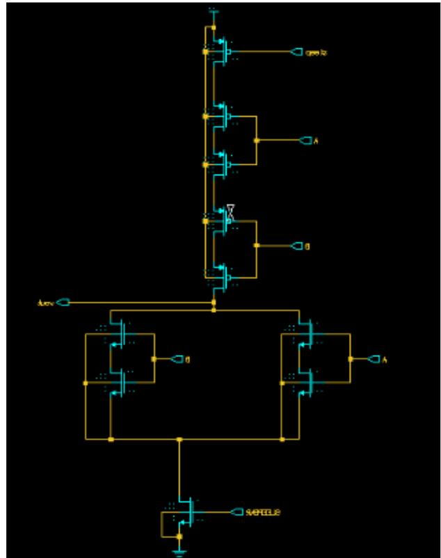
Fig. 9. NOR circuit using MTCMOS plus Stack technique
