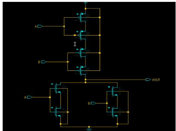
Fig. 6. Stack NOR circuit
