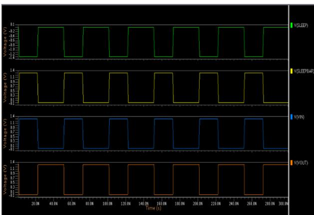
Fig. 13. Input-Output waveforms of Inverter circuit using MTCMOS plus Stack technique
