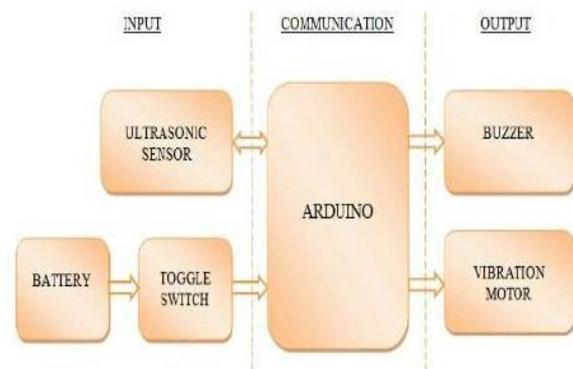
Fig 1: Block diagram of Existing Prototype
