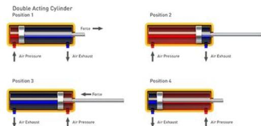
Figure 3: Double Acting Pneumatic Cylinder
