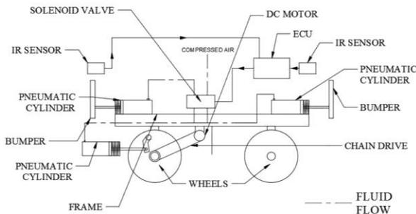
**Figure 5:** Construction Layout
