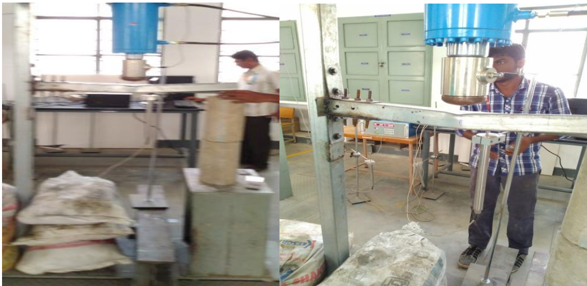
Figure 5. 1 & 5.2 Experimental set up for Z – Shaped cold formed steel sections( 110 x 45 x2 ), formed built up channel sections( 60 x 60 x4 ) mm)
