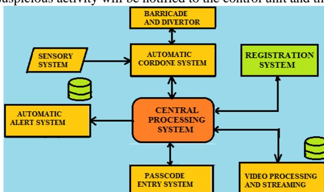
Figure 1: Automatic threat detection and response system
