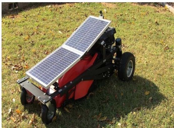
Figure 2: Smart Solar Grass Cutter With Lawn Coverage Source: http://www.robert-smith.net/my-projects/how-to-build-a-rc-lawn-mower/
