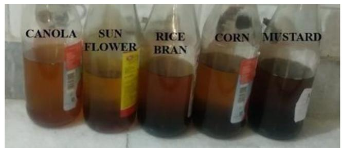
Fig. 5: Unseparated biodiesel from different oils.
