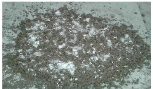
**Figure 3: Wet mix of materials with fibers added**
