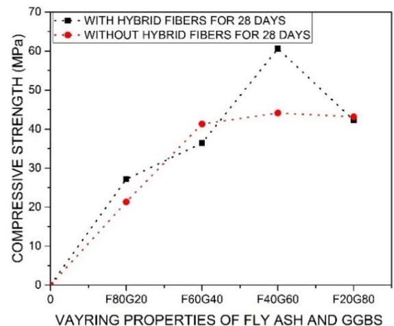
**Figure 5:** Compressive strength test results for 28 days curing of GPC with GGBS with hybrid fibers v/s without hybrid fibers in graph.
