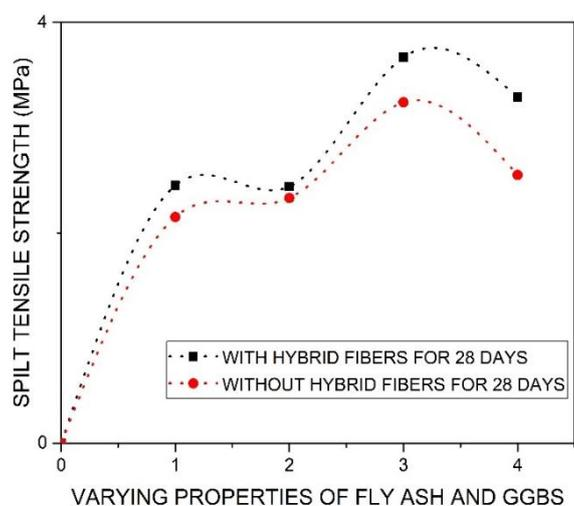
**Figure 7:** Split tensile strength test results for 28 days curing of GPC with GGBS with hybrid fibers v/s without hybrid fibers in graph.
