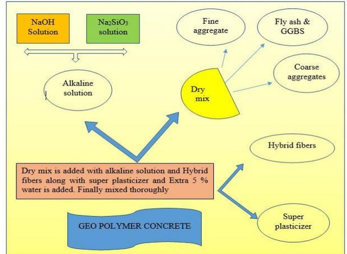
**Figure 1: Preparation detail of Geo polymer concrete**
