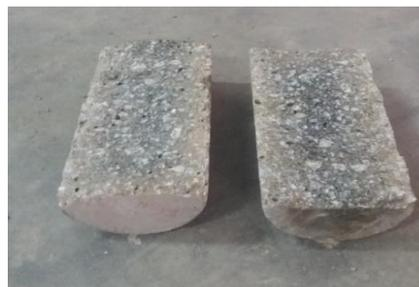
**Figure 6 :** Failed cylinder specimen under split tensile test
