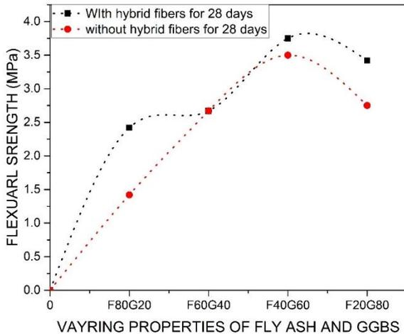
**Figure 8 :** Flexural strength test result for 28 days curing of GPC with GGBS and hybrid fibers v/s without fibers.
