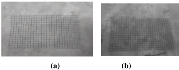
**Fig 1 (a) Weld mesh (b) Weld mesh with 2 layers of chicken mesh**
