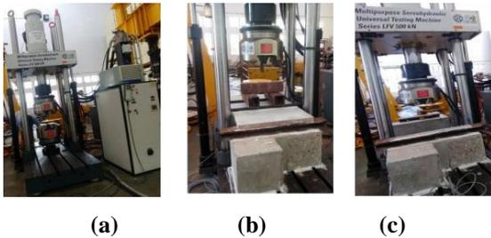
**Fig .3 (a) Testing machine (b) Flexural test setup (c) Test setup after placing slab**
