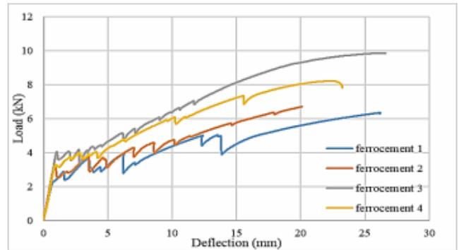
Fig.9 Result of Ferroceement panels
