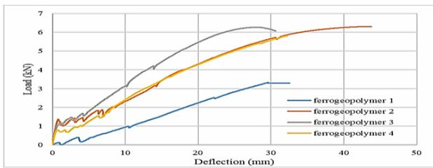
Fig.7 Result of geo-ferrocrete panels
