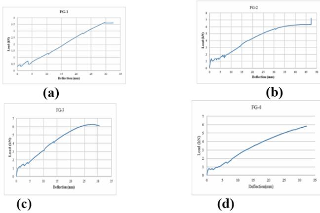
Fig.6 (a), (b), (c) and (d)-Load and deflection behaviour of Geo-ferrocrete panels
