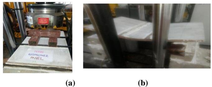
**Fig.5(a) Testing of geo-ferrocrete panel (b) Tested specimen**
