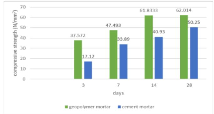
Fig.12 compressive strength test result
