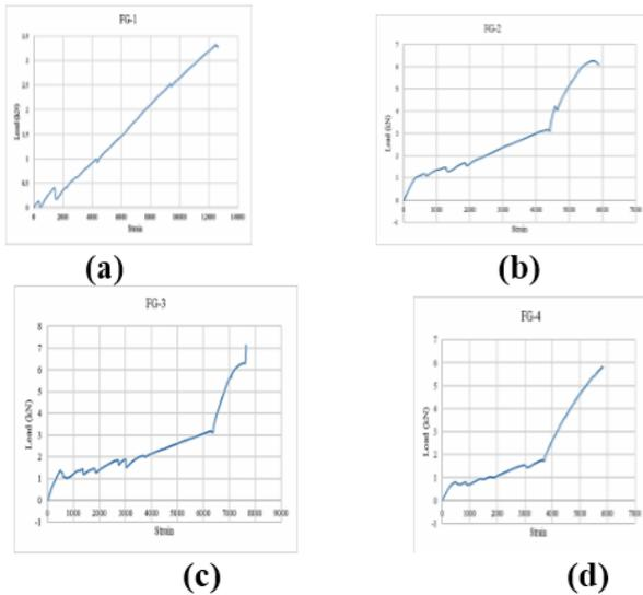
Fig.10 (a), (b), (c), (d) strain plot for geo-ferrocrete panels
