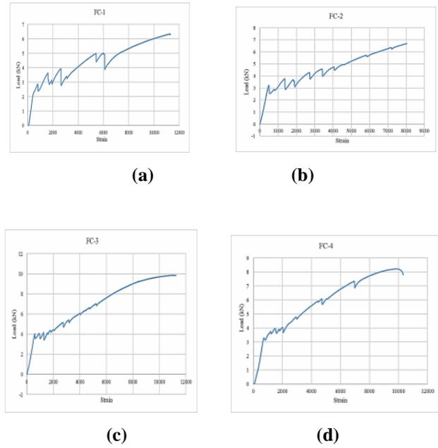
Fig.8 (a), (b), (c), (d)-Load and deflection behaviour of ferroceement panels
