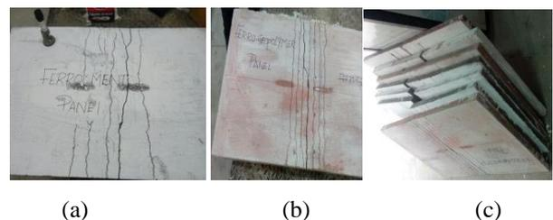
Fig.13 (a) cracking of ferrocement panel (b) cracking of ferro-gopolymer panel specimens after testing
