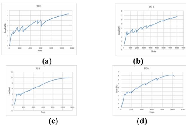
Fig.11 (a), (b), (c), (d) Strain behavior of Ferrocement panels
