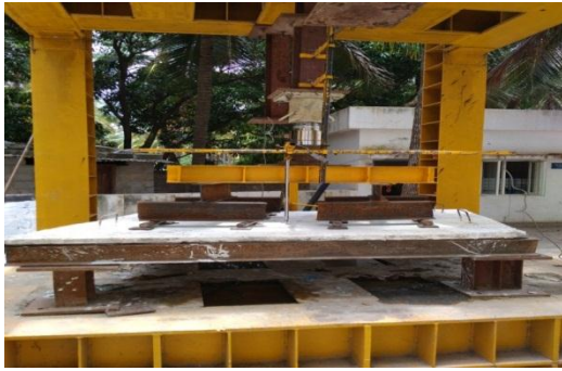
Figure 5: Testing of a Skew Slab under UDL
