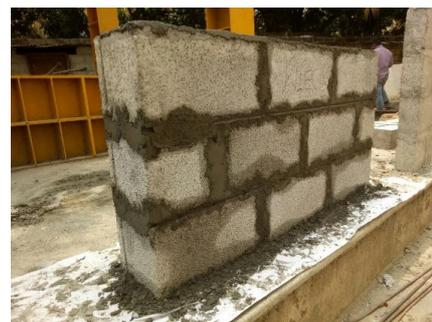
Fig -2: Masonry wallet after casting
