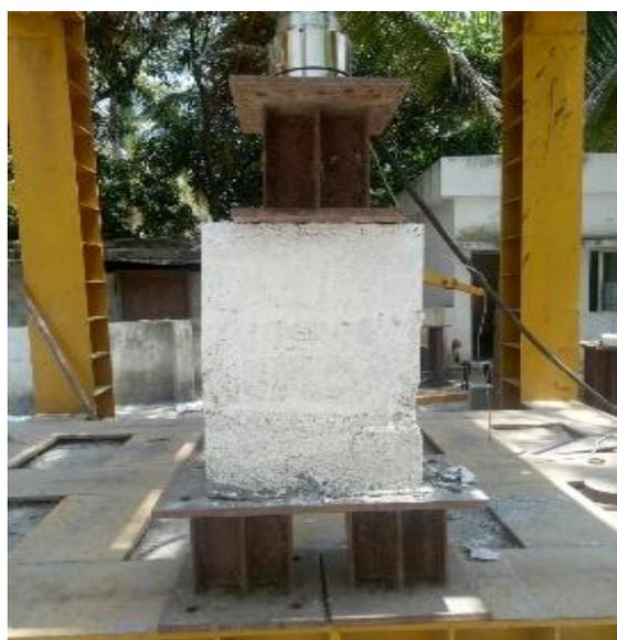
Fig-4 :Setup for Compression test
