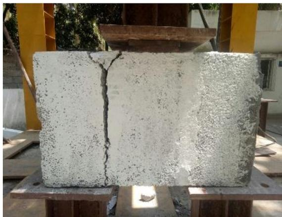
Fig -3: Setup for Shear test
