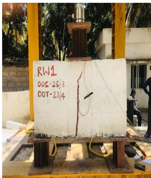
Fig -5: Setup for flexure test
