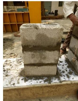
Fig -1: Masonry triplet Specimen after casting
