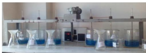
Figure 4: Jar test apparatus
