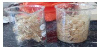
Figure 2: Combination of PVA and bagasse
