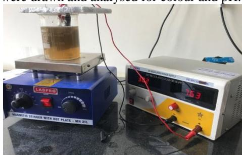
Fig 3: Experimental Set Up of Electrochemical Oxidation Process
