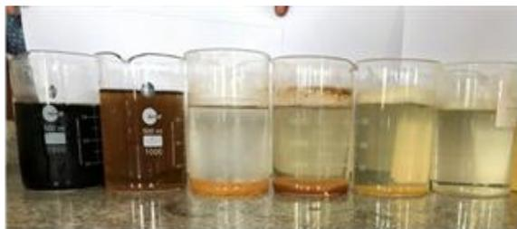
Fig 5: Sample Before and After Treatment for various current densities.
