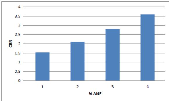
**III. Effect of molasses & areca nut fibers on strength properties of BCS**
