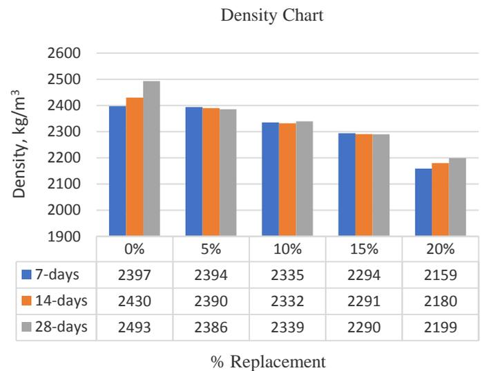
**Figure 1.** Density test on concrete
