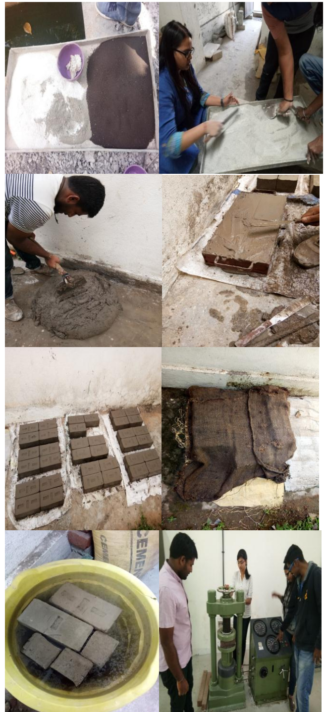
Plate 1: Various stages of preparing, stacking, numbering, curing and testing adobe blocks
