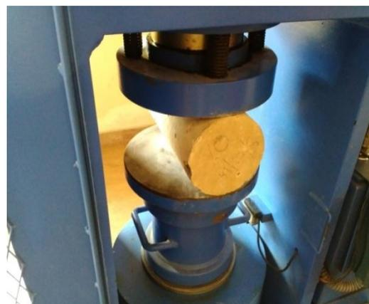
**Figure 2** Split Tensile Testing
