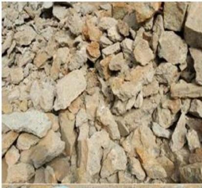
Figure 1: Crushed waste concrete
