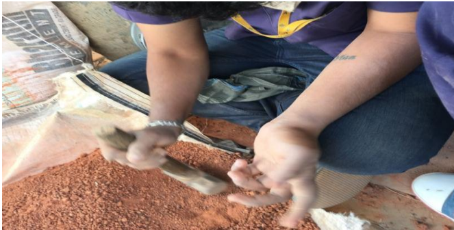
Figure 1: Process of making brick powder
