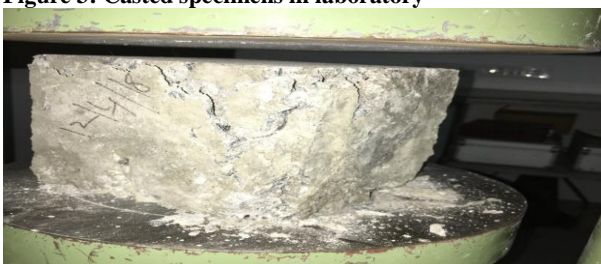
Figure 4: Failure patterns of specimens
