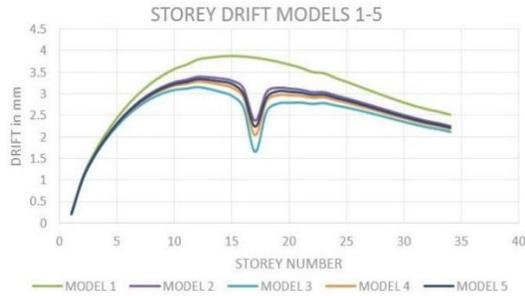
**Fig. 5:** Storey drift for models 1-5
