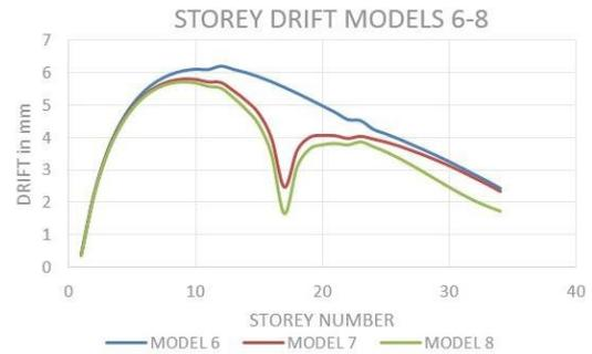
**Fig. 7:** Storey drift for models 6-8
