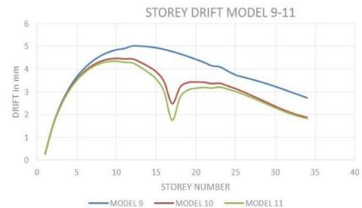
**Fig. 9:** Storey drift for models 9-11
