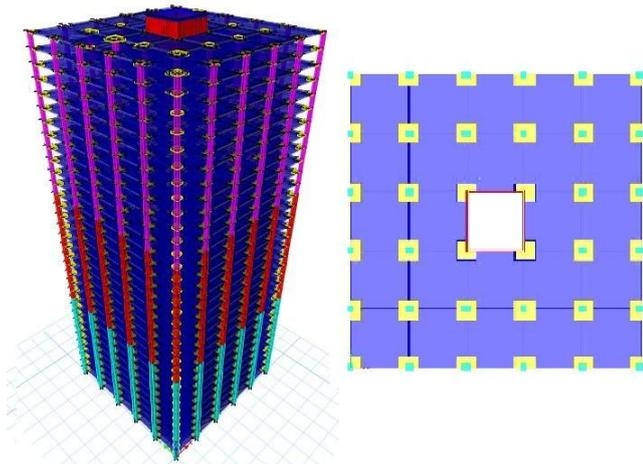
Fig. 3: 3D and 2D view of ETabs model
