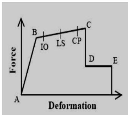
Figure 2: Typical force deformation curve
