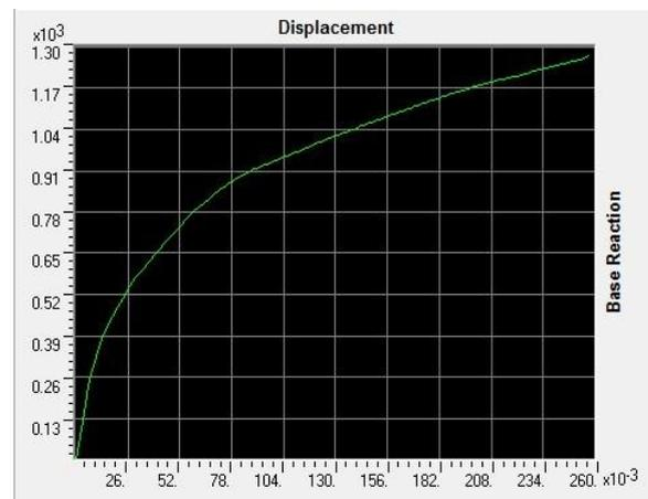
**Figure 6:** Displacement (m) vs. Base Shear (kN)
