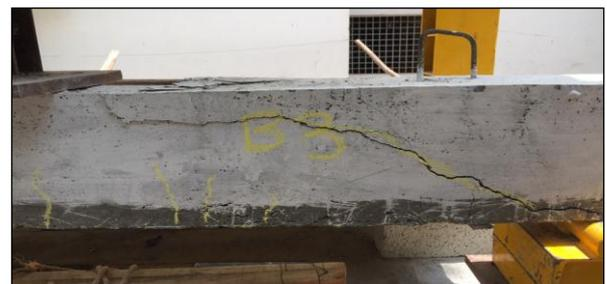
**Figure 6: Shear failure at the support**
