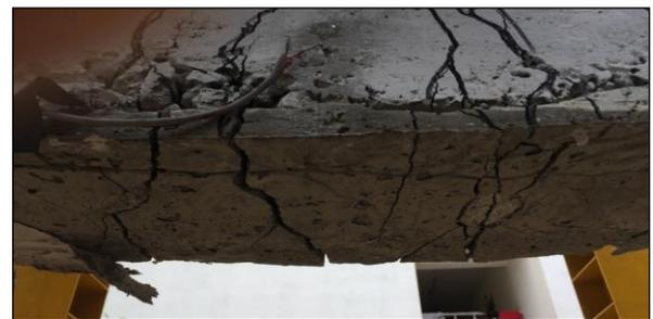
**Figure 5: Crack pattern after failure**
