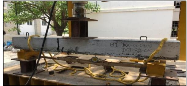
**Figure 3: Specimen setup for testing on loading frame**
