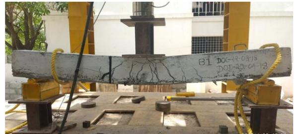
**Figure 4: During ultimate loading – Plastic hinge rotation**
