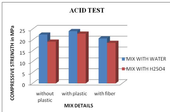
**Figure 6** percentage loss in compressive strength due to acidity
