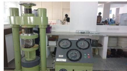
**Figure 1** Compression testing machine
