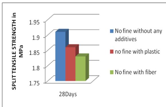
Figure 4 Split tensile strength of no-fine concrete cylinder
