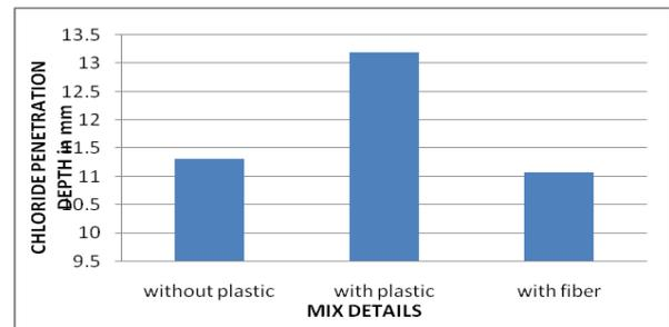
Figure 5 Depth of chloride Penetration in no-fine concrete mix
