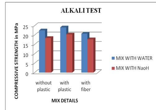
**Figure 7** percentage loss in compressive strength due to alkalinity
