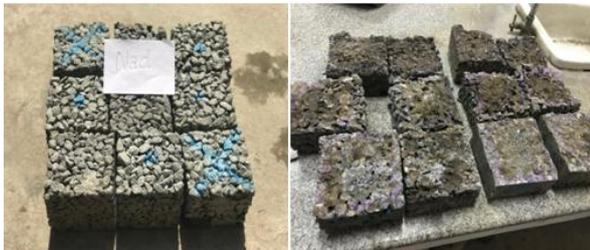
**Figure 2** Typical Chloride Penetration Depth after 28 Days Exposure
