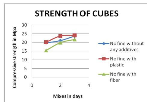
**Figure 3** Compression strength of no-fine concrete cubes with different additives
