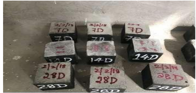
Figure 2: Cement mortar cubes
