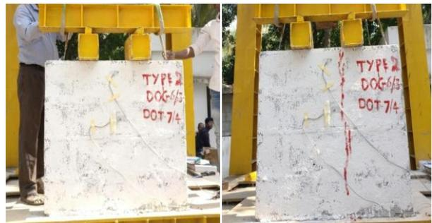
**Figure 5:** Test setup of block masonry wall Type 2 before and after testing for compression strength.
