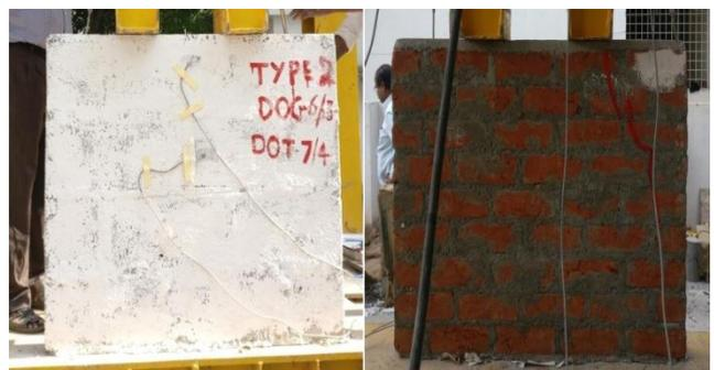
**Figure.7:** Test setup of brick masonry wall Type 2 before and after testing for compression strength.
