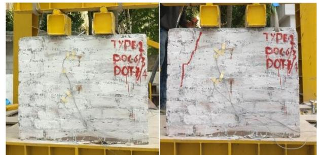
**Figure. 6:** Test setup of brick masonry wall Type 1 before and after testing for compression strength.
