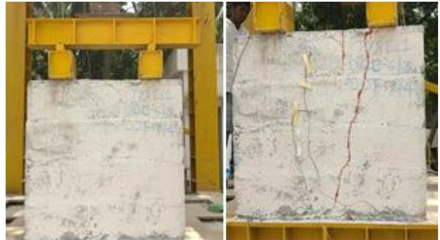
**Figure 4:** Test setup of block masonry wall Type 1 before and after testing for compression strength.
