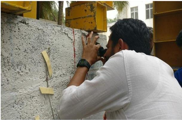
**Figure 8:** Measuring crack width using Travelling Microscope
