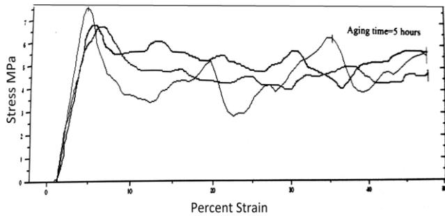
Fig.4. Compressive behavior of foam samples with 0.15 R.D. and aging time 5 hours.
