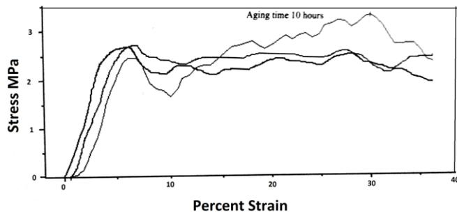
Fig.5. Compressive behavior of foam samples with 0.15 R.D. and aging time 10 hours.
