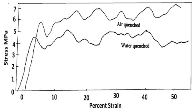
Fig.3. Compressive behavior of foam samples with R.D=0.2, solutionized at 505°C for 1 hour followed by air or water-quenching.
