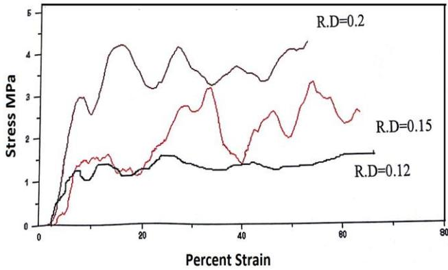
Fig.1. Compressive behavior of as foamed foam samples with different relative densities.
