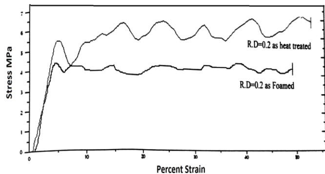
Fig.2. Compressive behavior of foam samples with 0.20 R.D. heat treated and as foamed.
