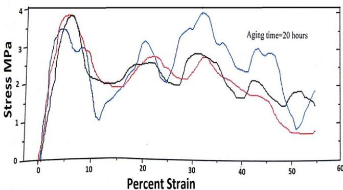
Fig.6. Compressive behavior of foam samples with 0.15 R.D. and aging time 20 hours.
