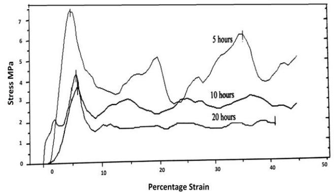
Fig.7. Compressive behavior of foam samples with R.D.=0.15 heat treated air quenched 5 hours, 10 hours and 20 hours.
