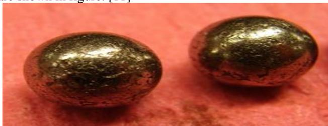
Fig. 1 Pitting on ball bearing elements
