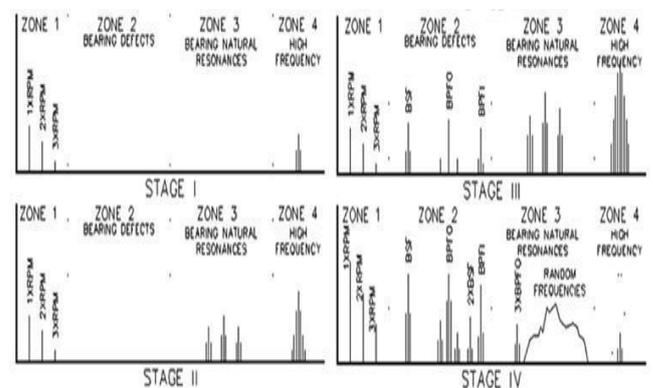
Fig. 4 Progression of defect in bearing
