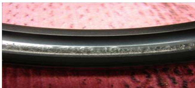
Fig. 3 Spalling on Outer race
