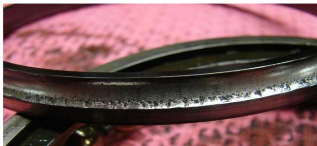
Fig. 2 Spalling on Inner race
