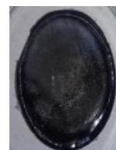
Fig. 1c Thin Film of Polyaniline Coated Glass Fiber
