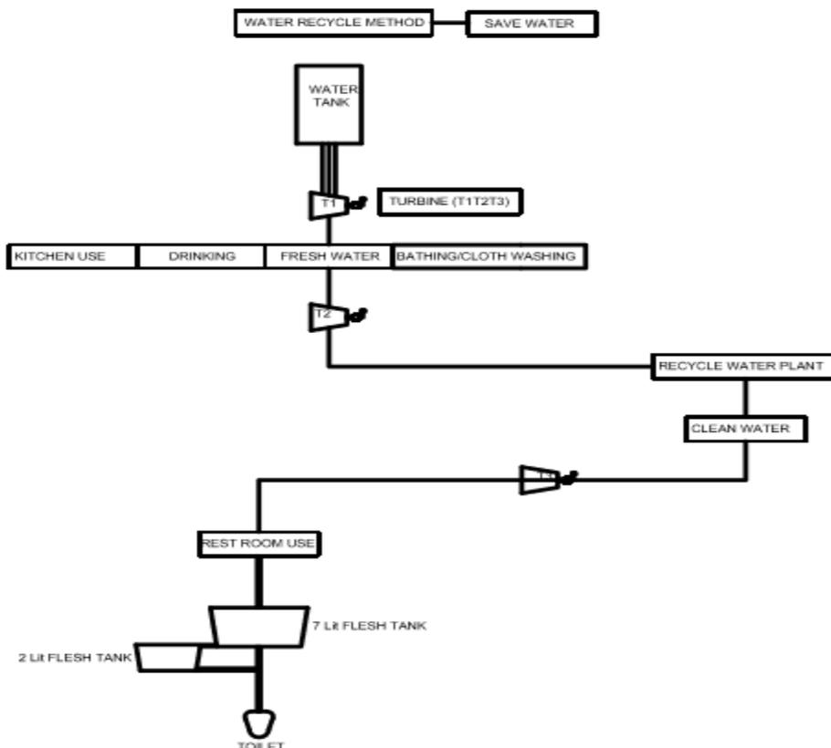
**Figure 1. Water re-cycle layout.**
