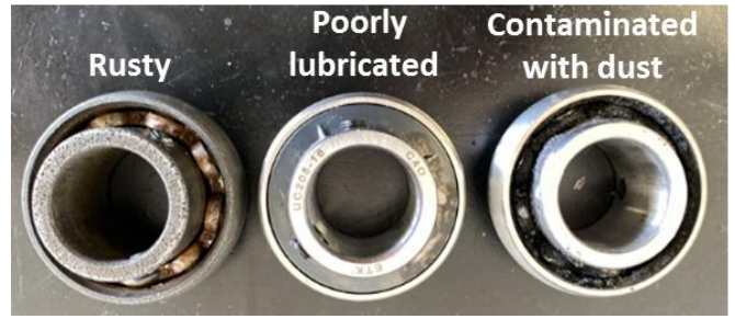
Figure 6. Bearings for inspection
