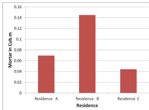
**Figure 2.** Comparative analysis of quantity of cement sand mortar used for brickwork and wall plastering per Sq.M area of each residence
