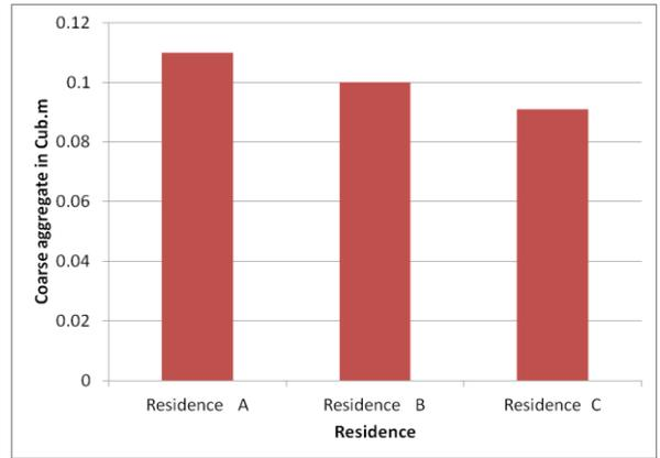
**Figure 5.** Comparative analysis of quantity of coarse aggregate used for roof work per sq.m area of each residence
