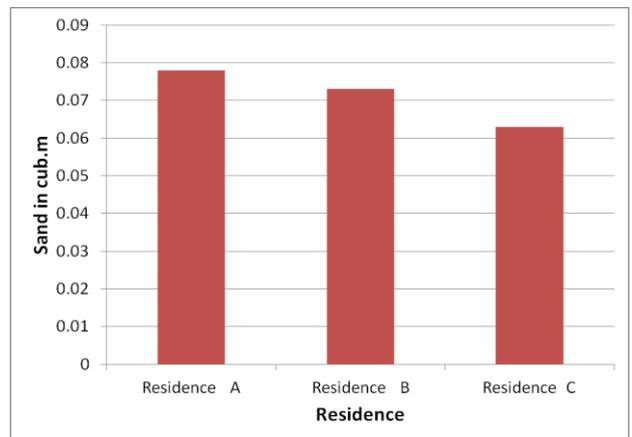
**Figure 7.** Comparative analysis of quantity of sand used for roof work per sq.m area of each residence
