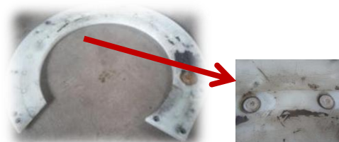
Figure 1. Damaged starwheel's baseplate
