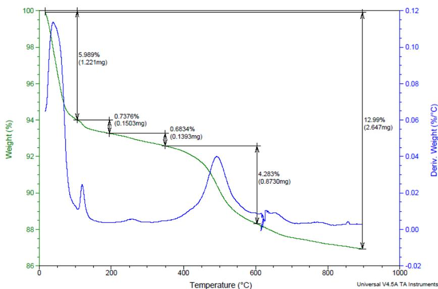
**Fig (3)** TGA Pattern for Clay
