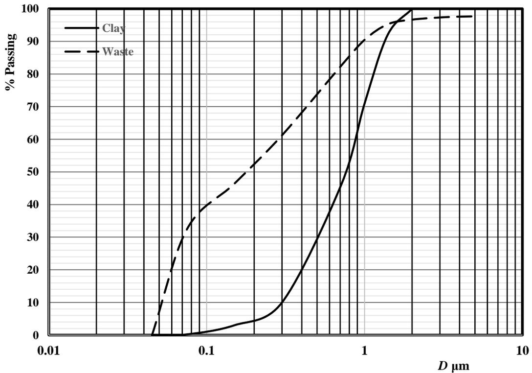
**Fig (5)** Cumulative screen analysis of raw materials
