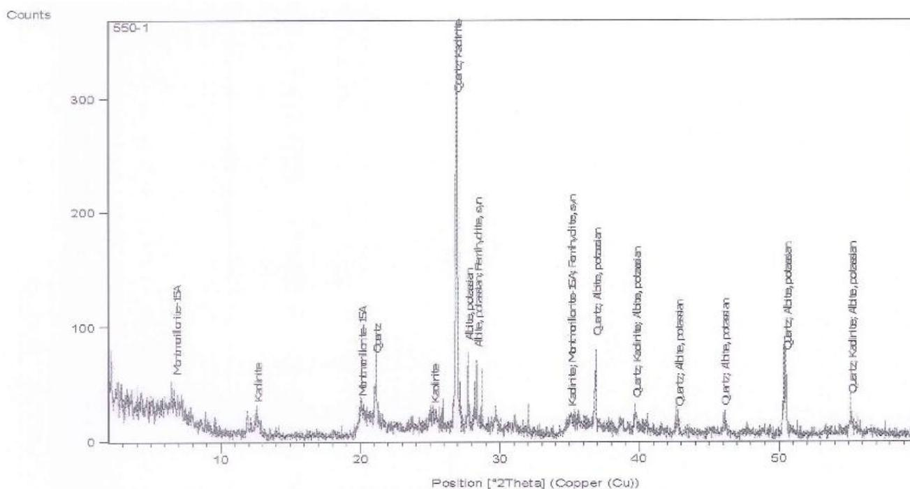
**Fig (1)** XRD Pattern for Clay
