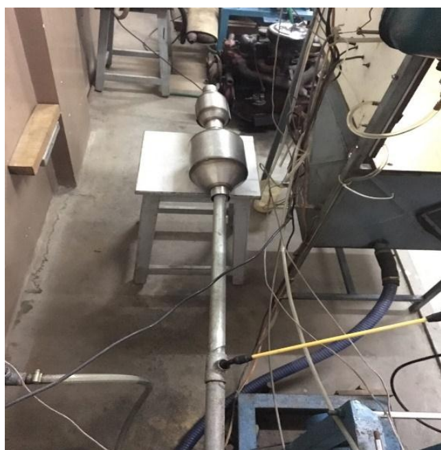
Fig 2. Photograph of DPF, DOC & Injecting Hydrazine Hydrate at exhaust pipe
