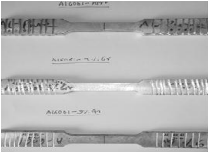
Figure 5: Tensile specimens of base MMCs
