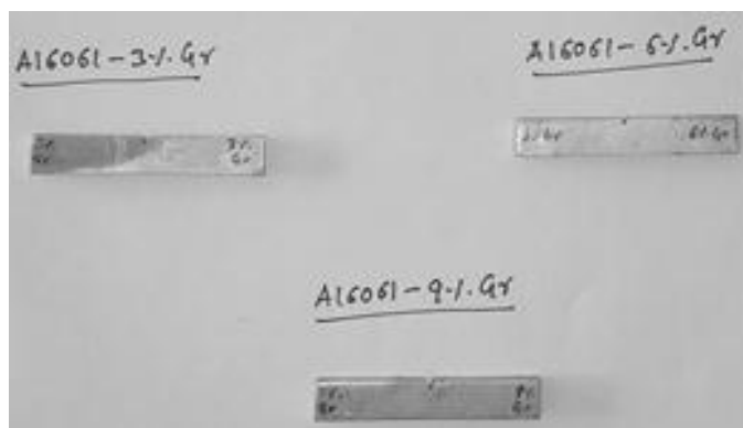
Figure 16: Charpy specimens of base MMCs
