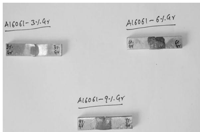
Figure 17: Charpy specimens of microwave weld MMCs
