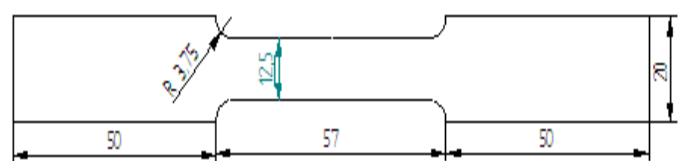
Figure 4: Tensile test specimen dimensions (mm)
