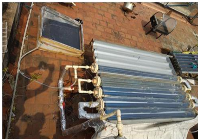
Fig. 2: Solar still coupled with CPC Arrangement
