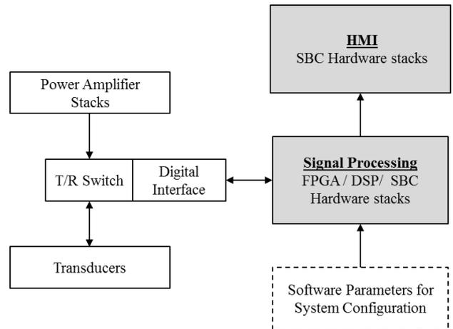
Fig. 1. Typical SDS system configuration
