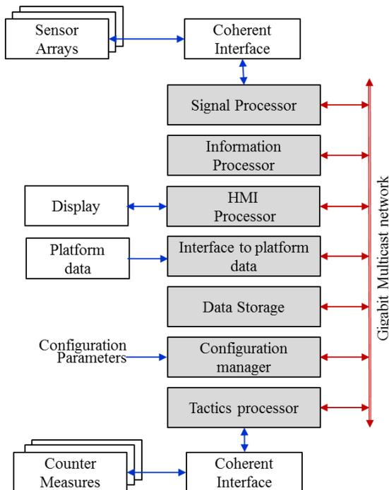
**Fig. 5** Networking and data Communication scheme
