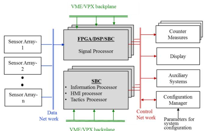
Fig. 4 Hardware configuration for TDS with SDS architecture
