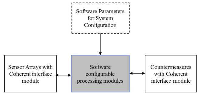
Fig. 3 Hardware modules for TDS with SDS architecture
