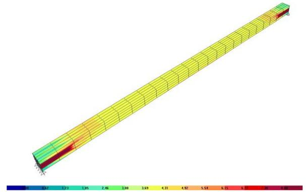
**Figure 6a:** Normal stress on *Brick* elements of the reinforced tie beam, in the direction of its axis
