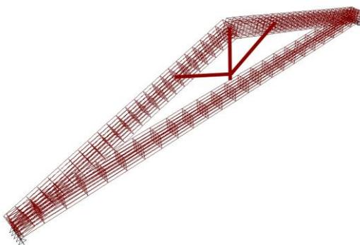
**Figure 2a:** Undeformed configuration of the truss with *Brick* and *Frame* elements
