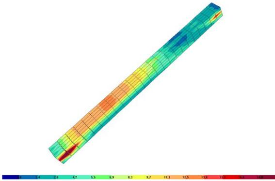
**Figure 7b:** Von Mises stress on *Brick* elements of the reinforced rafter
