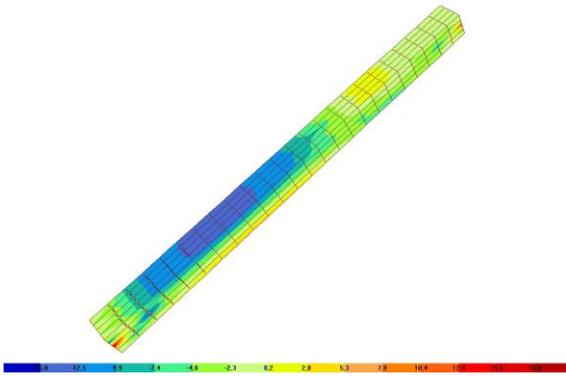
**Figure 4b:** Normal stress on *Brick* elements of the rafter, in the direction of its axis
