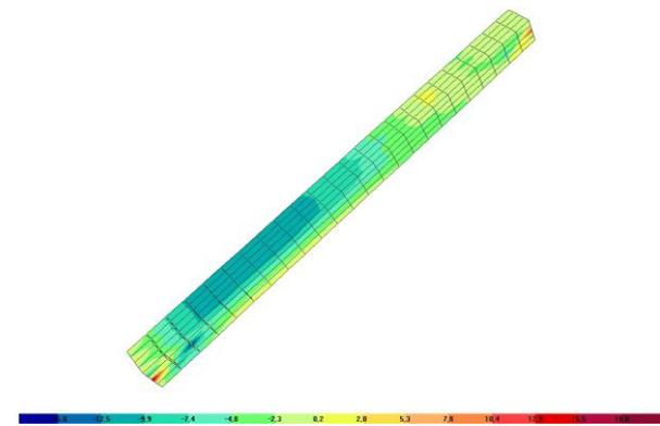
**Figure 6b:** Normal stress on *Brick* elements of the reinforced rafter, in the direction of its axis
