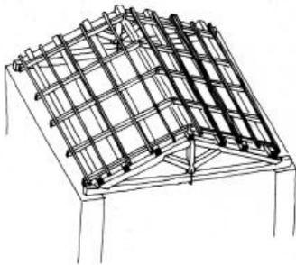
**Figure 1:** The classic wooden roofing pattern widely used in Northern Italy
