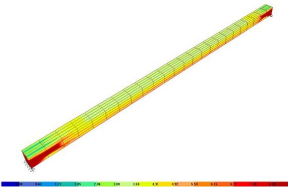
**Figure 5a:** Von Mises stress on *Brick* elements of the tie beam
