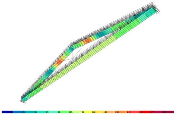
**Figure 8:** Von Mises stress distribution within the reinforcement fabrics only
