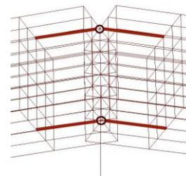
**Figure 3b:** Connection model of the rafters to each other
