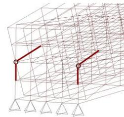
**Figure 3a:** Connection model between the rafter and the tie beam
