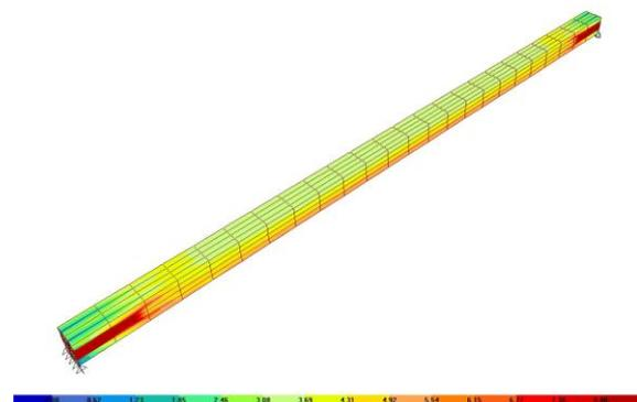
**Figure 4a:** Normal stress on *Brick* elements of the tie beam, in the direction of its axis
