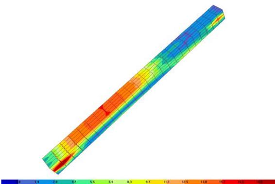
**Figure 5b:** Von Mises stress on *Brick* elements of the rafter
