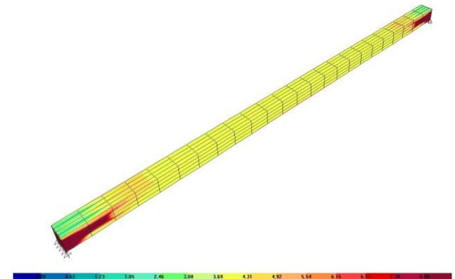
**Figure 7a:** Von Mises stress on *Brick* elements of the reinforced tie beam
