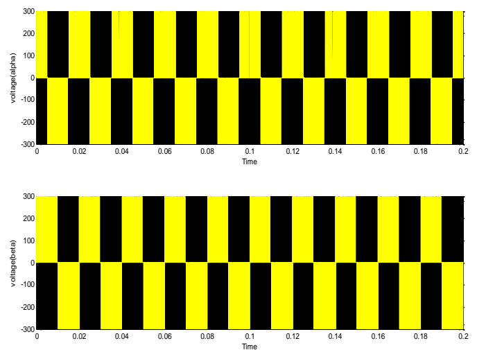
Fig. 6: Two phase output from three leg inverter
