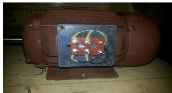
Fig.18: Fabricated two phase symmetrical motor (Rating 1.3H.P.1000 rpm)
