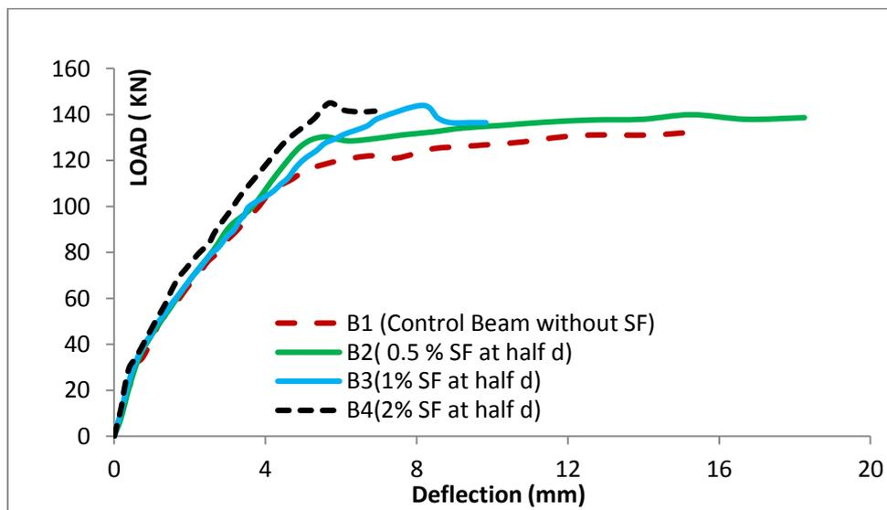
Figure 8. Load deflection curve for specimens with different steel fiber ratios at half depth
