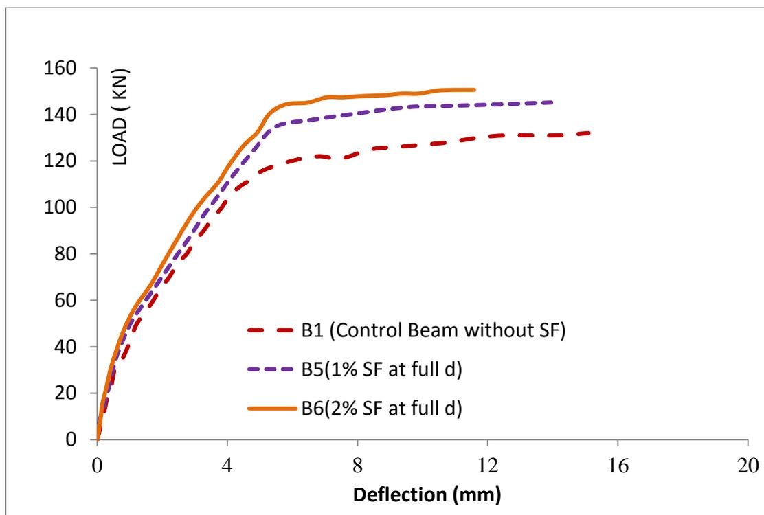
**Figure 9.** Load deflection curve for specimens with different steel fiber ratios at full depth
