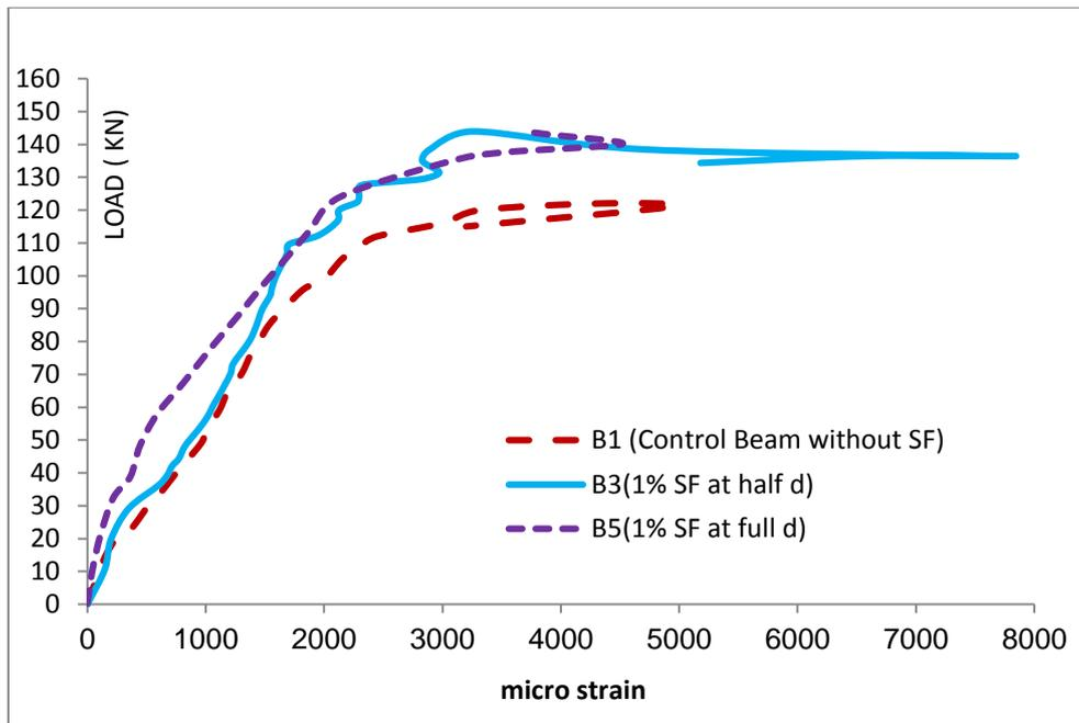
**Figure 18.** Load strain curve for specimens with a 1% steel fiber ratio at half and full depths
