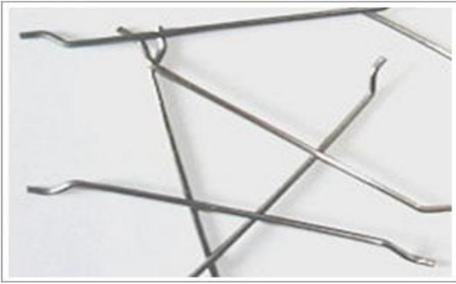
Figure 1. Hooked-end shaped steel fiber used in this study
