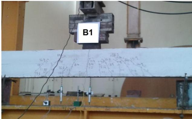
**Figure 4.** Test setup and LVDT arrangement
