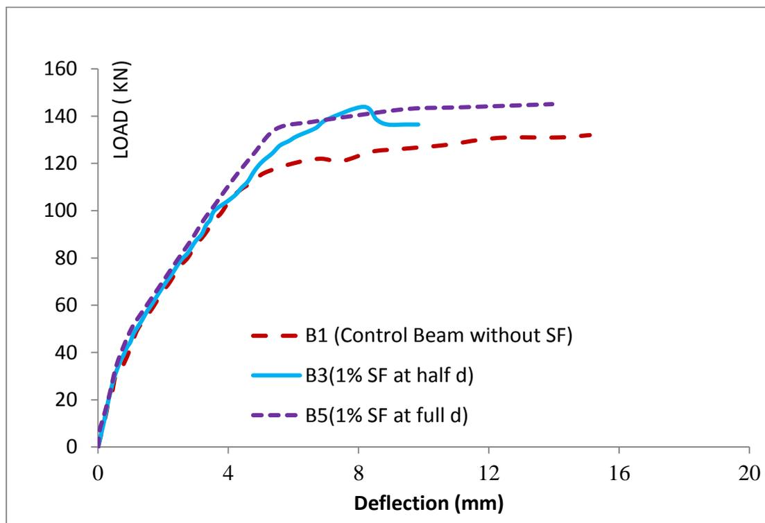
**Figure 10.** Load deflection curve for specimens with a 1% steel fiber ratio at half and full depths
