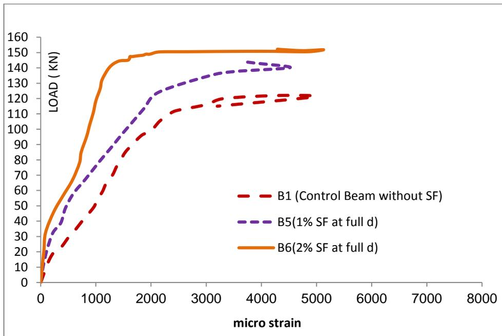
**Figure 17.** Load strain curve for specimens with different steel fiber ratios at full depth
