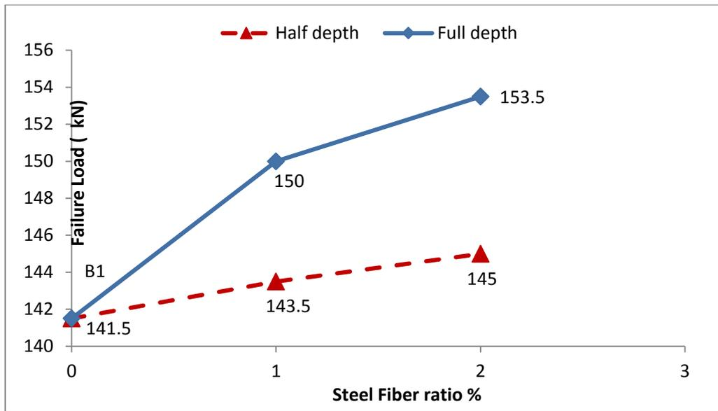
Figure 7. Influence of the steel fiber distribution depth and ratios on the failure load.
