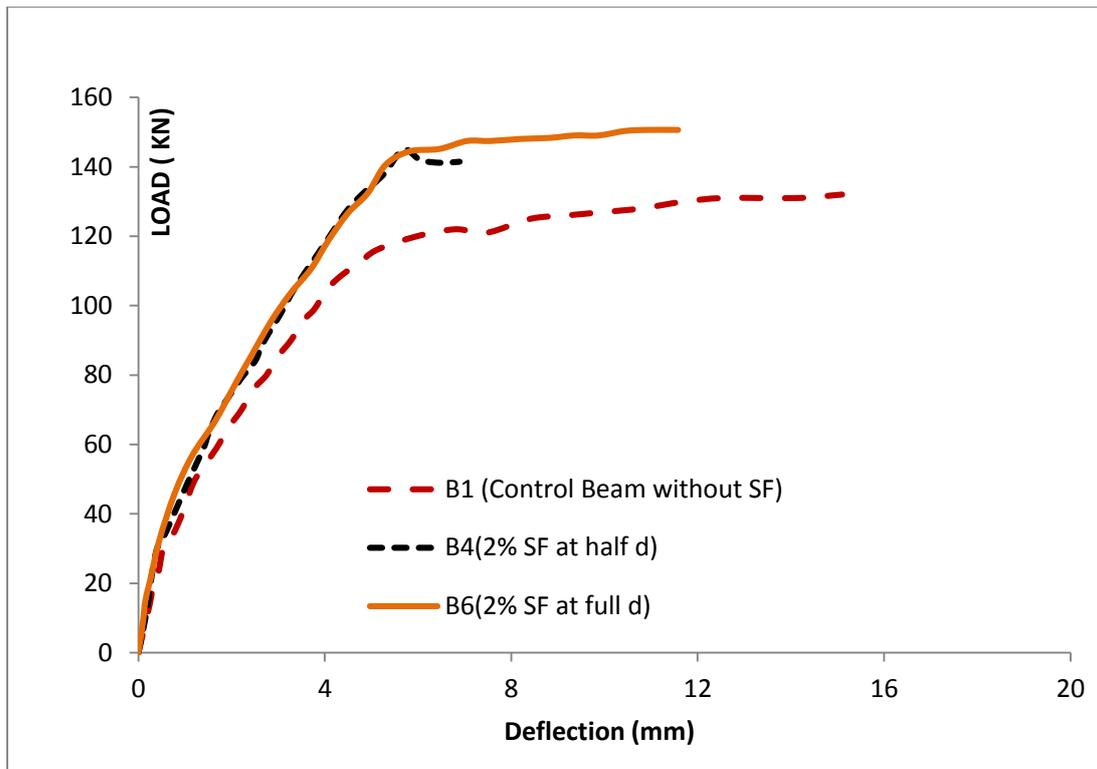
**Figure 11.** Load deflection curve for specimens with a 2% steel fiber ratio at half and full depths
