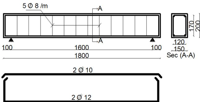
Figure 2. Typical beam specimen dimension and reinforcement details
