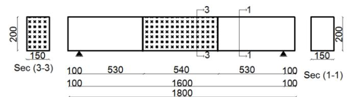
c. Beams B4 and B6 details
