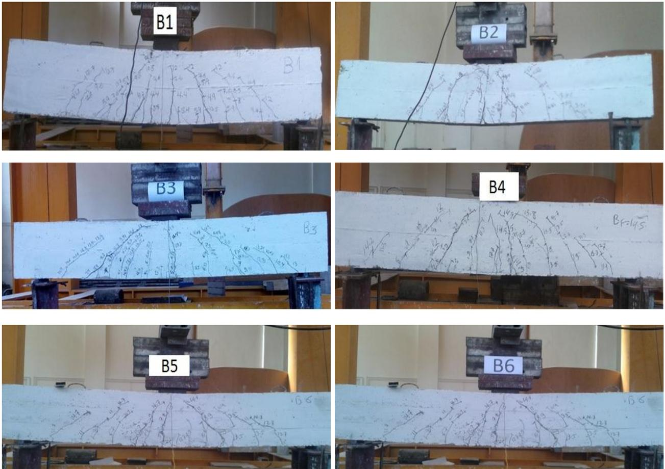
**Figure 5.** Failure mode of all tested specimen beams
