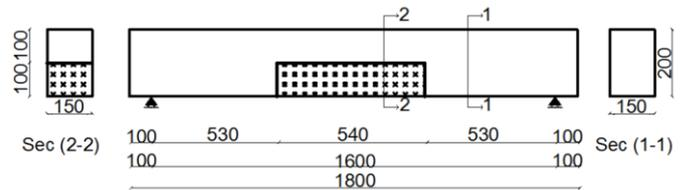
b. Beams B2, B3, and B5 details
