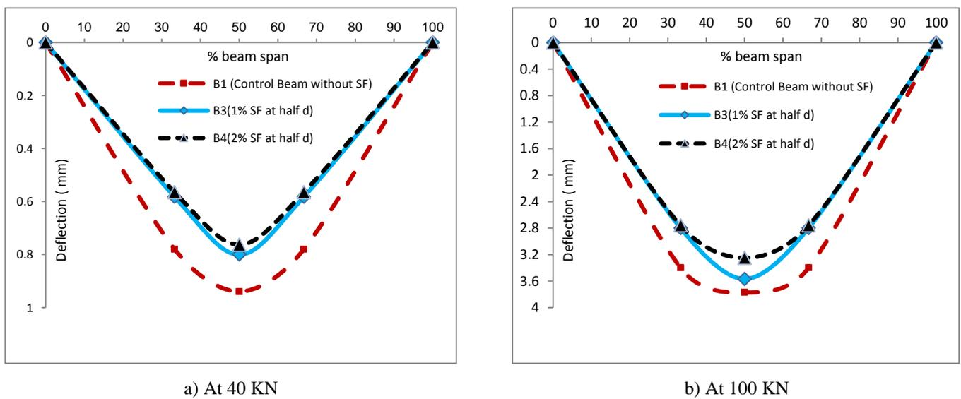
**Figure 12.** Beam deformation shape with a different steel fiber ratios at half depth
