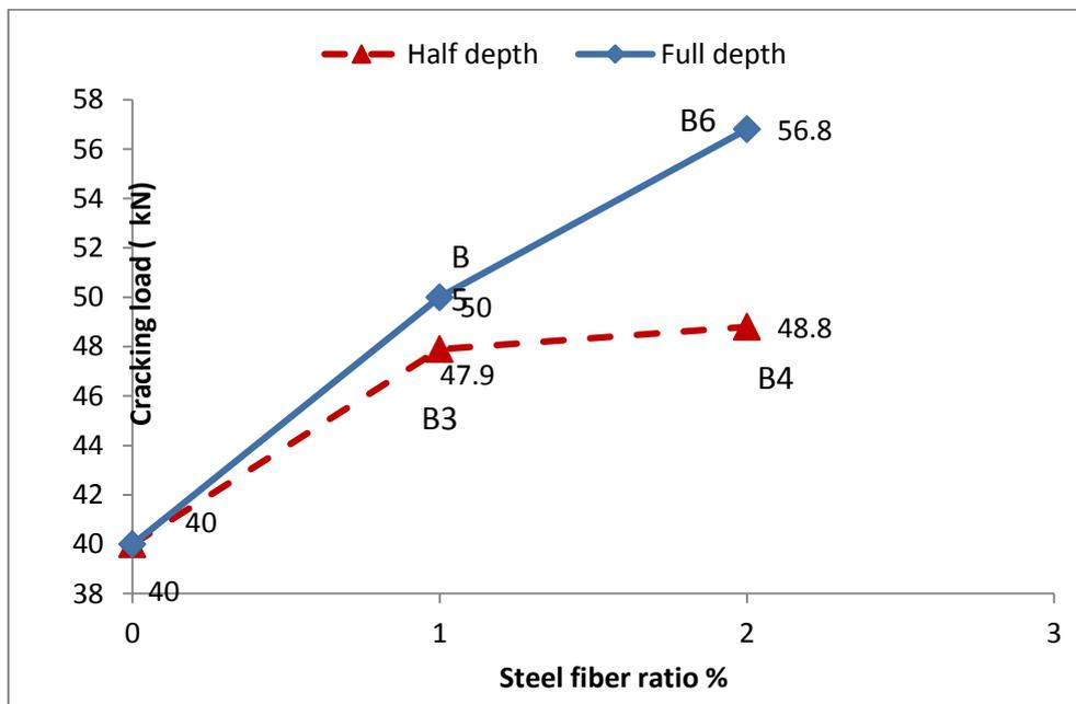
**Figure 6.** Influence of the steel fiber distribution depth and ratios on the cracking load.
