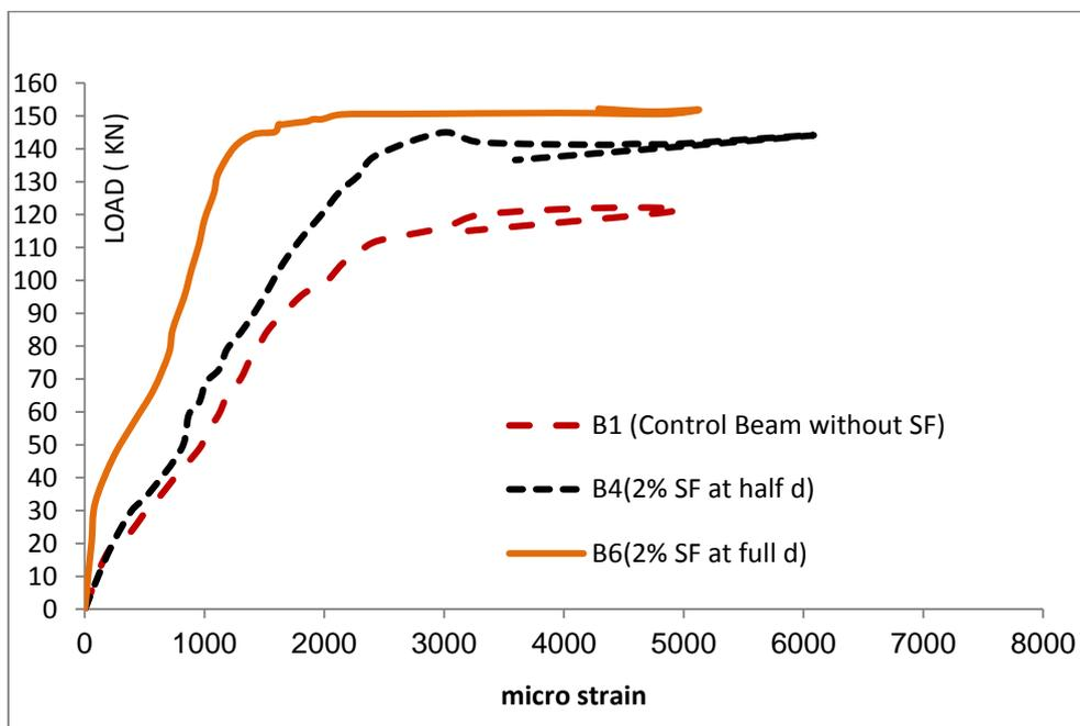
**Figure 19.** Load strain curve for specimens with a 2% steel fiber ratio at half and full depths
