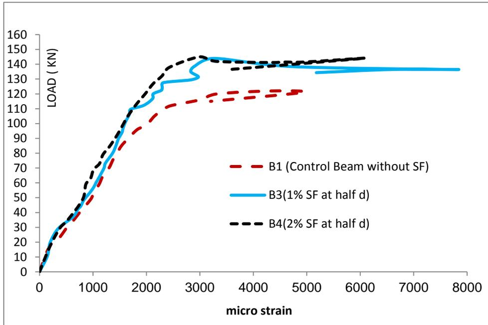
**Figure 16.** Load strain curve for specimens with different steel fiber ratios at half depth
