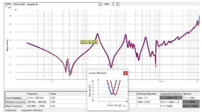
**Figure 10.** SFRA LVU-N OC Inductive measurement
