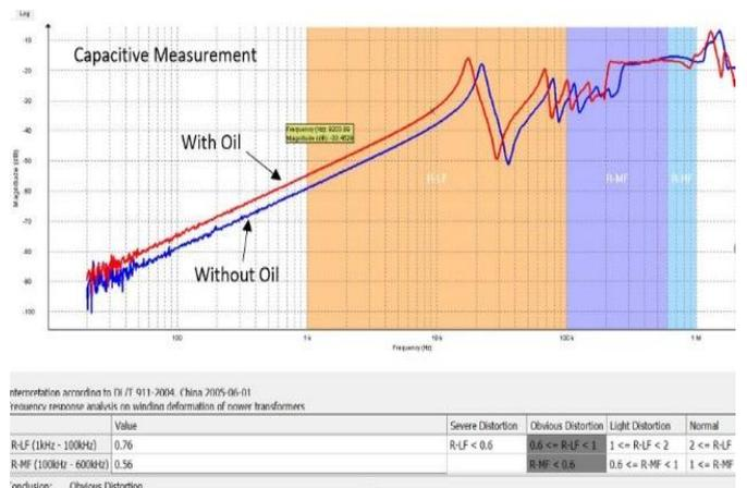
Figure 5. SFRA capacitive measurement comparison
