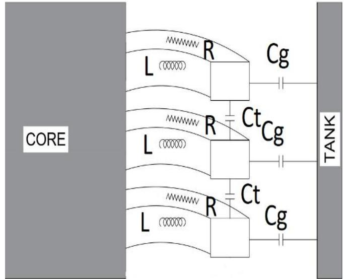
Figure 1. R, L and C of Transformer.
