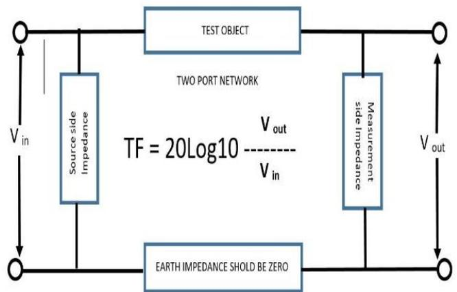
Figure 2. Power Transformer as a two-port network
