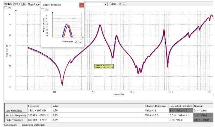
**Figure 9.** SFRA HVU-N OC Inductive Measurement
