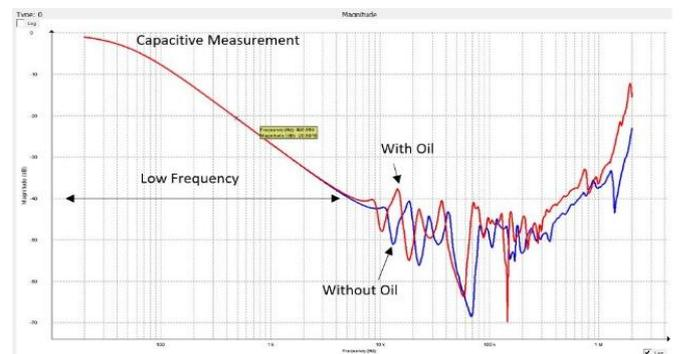
Figure 8. SFRA HVR-B SC Capacitive measurement
