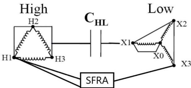
**Figure 4.** SFRA Capacitive measurement
