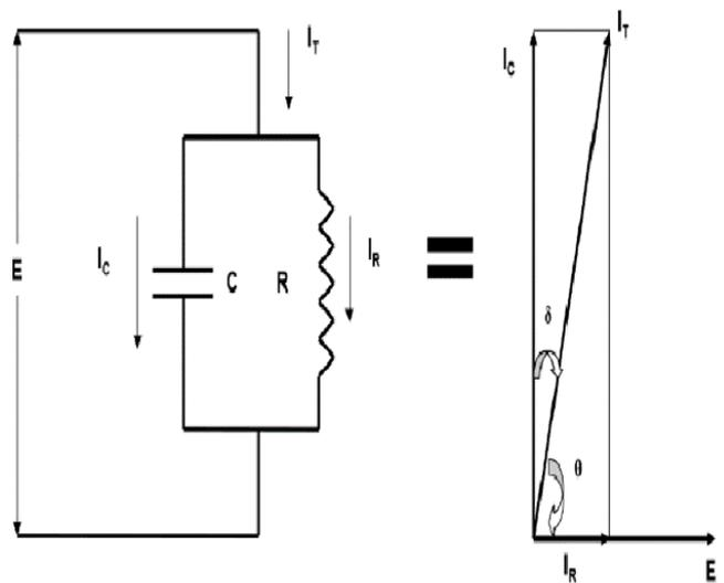
**Figure 4.** Tan Delta test principle
