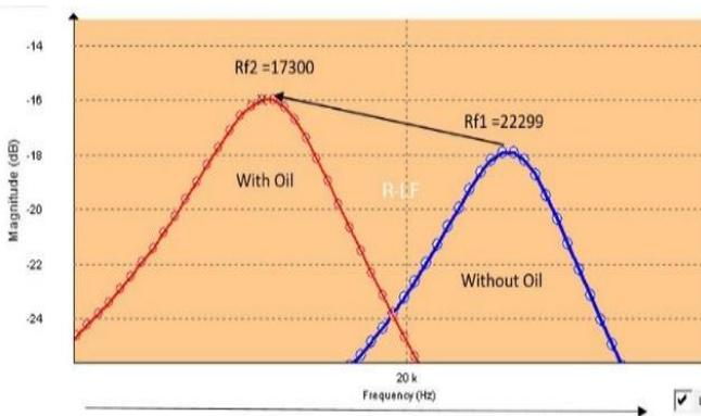
Figure 6. Shift in resonance due to absence of oil
