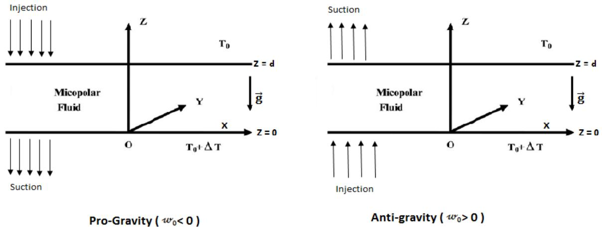
**Figure 1:** Schematic Diagram of the Flow Configuration
