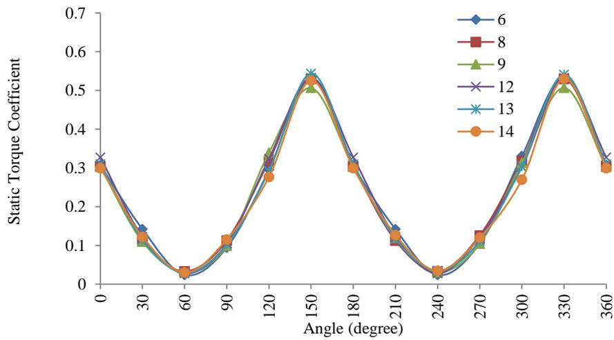
**Figure 20.** Static torque coefficient variation with angle of rotation for two blade IceWind turbine
