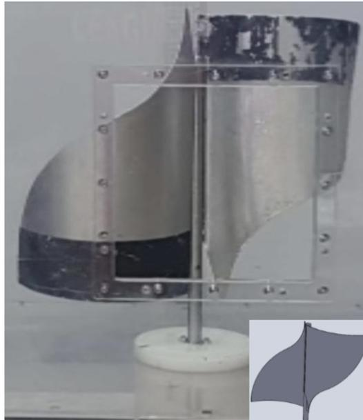
**Figure 7.** A photograph of tested two reversed blade IceWind turbine
