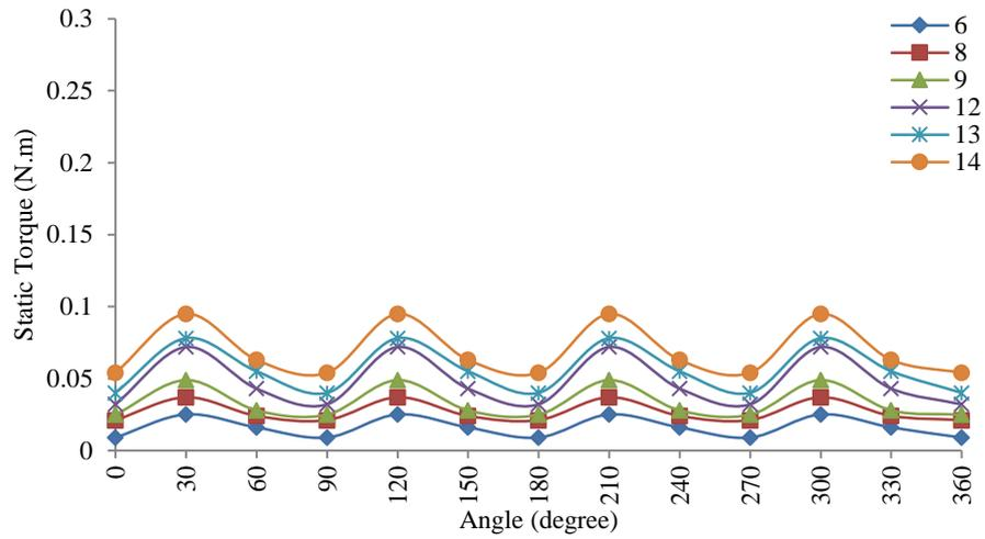
**Figure 19.** Static torque variation with angle of rotation for four blade IceWind-turbine.
