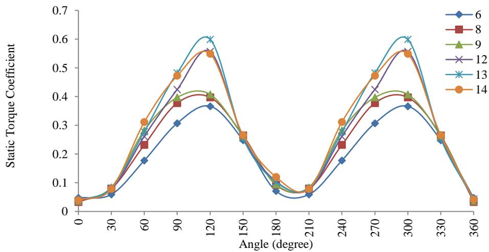
**Figure 21.** Static torque coefficient variation with angle of rotation for two-reverse blade IceWind turbine.
