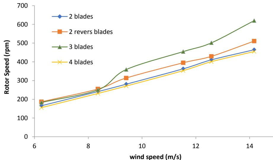
Figure 14. The rotor rotational speed (rpm) versus wind speed (m/s) for two, two-reverse, three and four blade IceWind turbines
