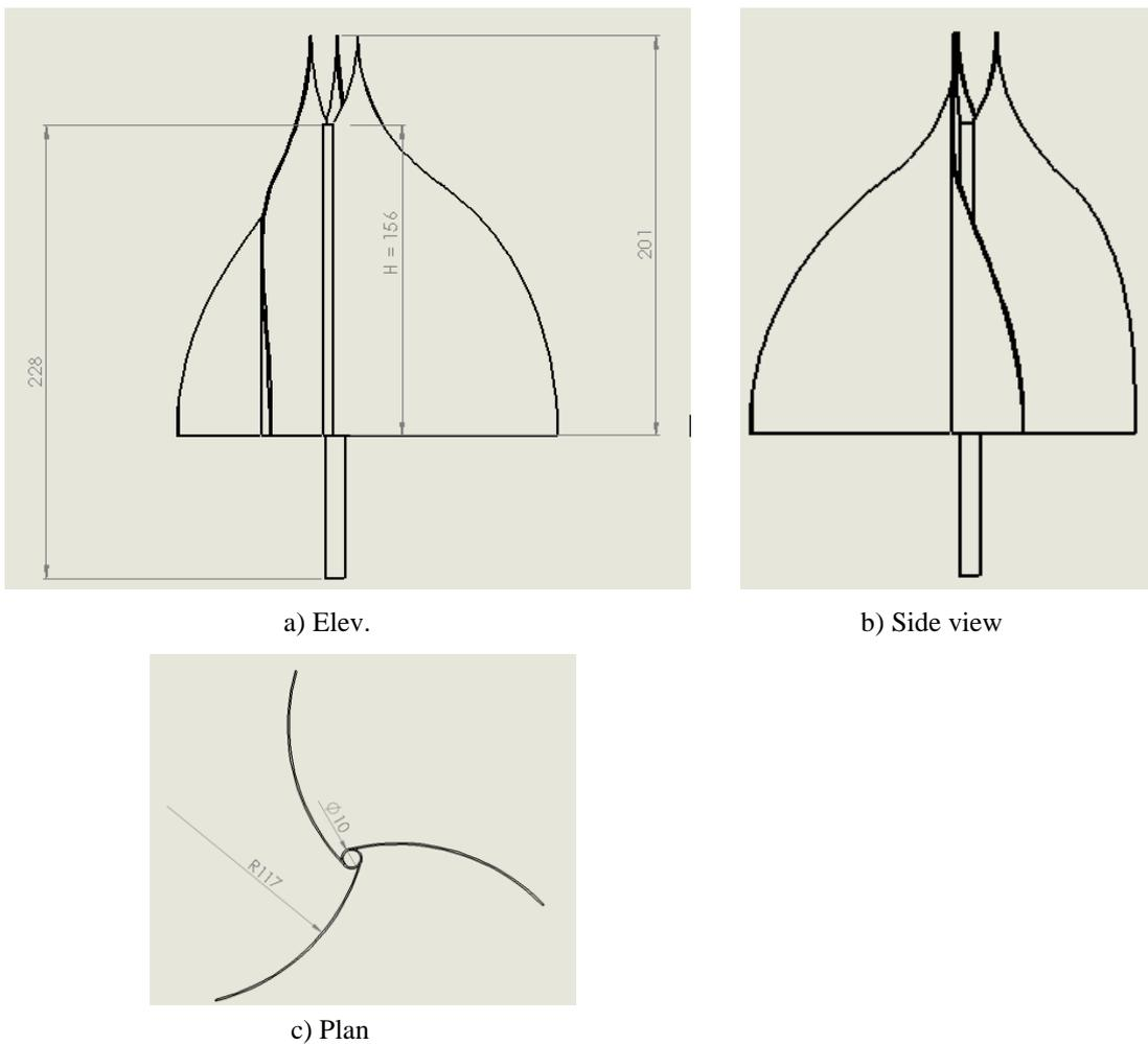
**Figure 10.** Three blade IceWind turbine's three views (Dimensions in mm)
