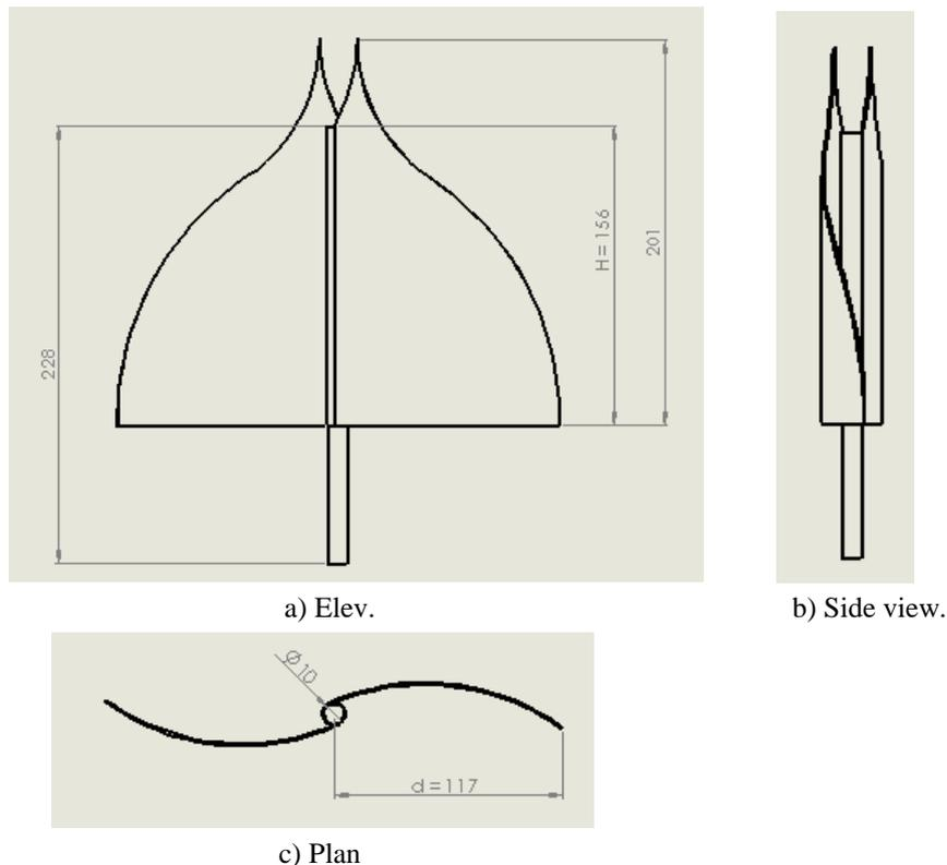
**Figure 6.** Two blade IceWind turbine's three views (Dimensions in mm)
