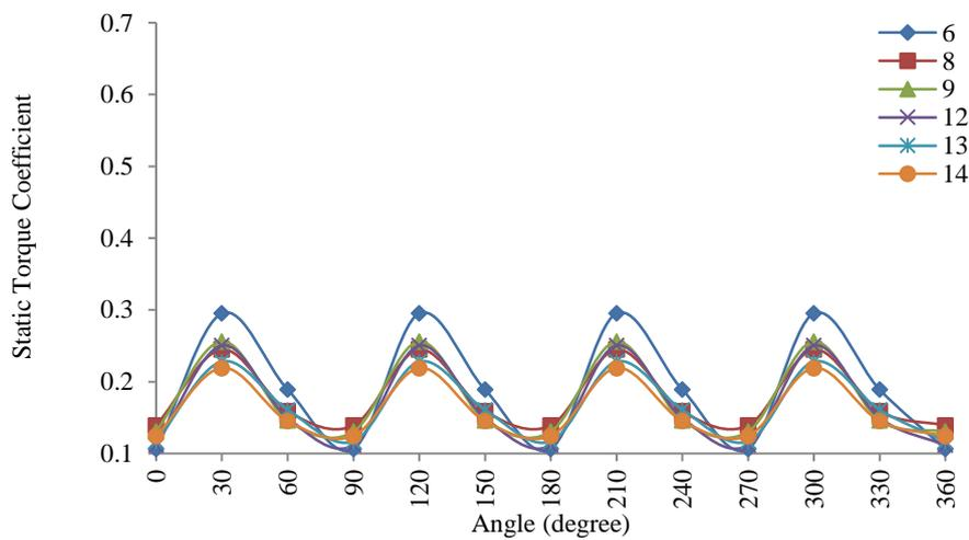
**Figure 23.** Static torque coefficient variation with angle of rotation for four blade IceWind turbine
