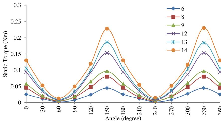
**Figure 16.** Static torque variation with angle of rotation for two blade IceWind-turbine.
