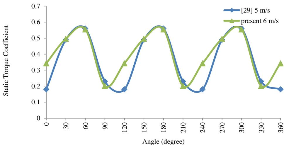
**Figure 25.** Comparison between three blade IceWind and three blade Savonius turbines using static torque coefficient variation with angle of rotation
