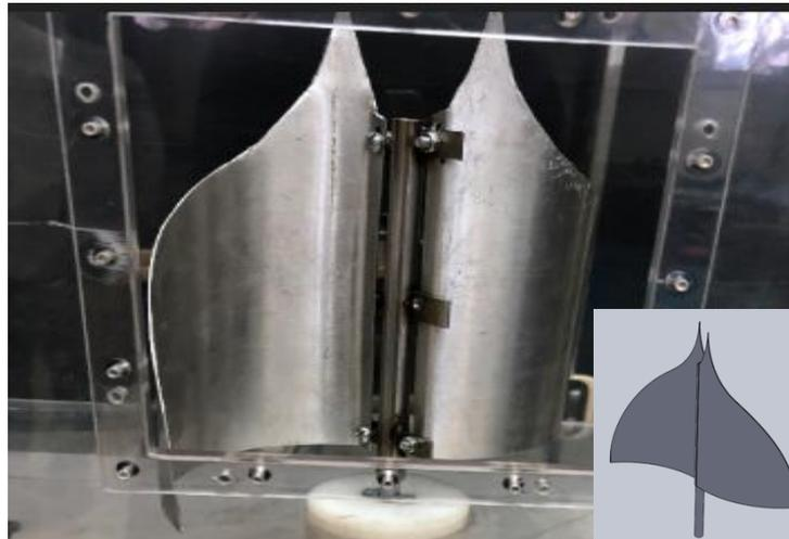
**Figure 5.** A photograph of tested two-blade IceWind turbine.
