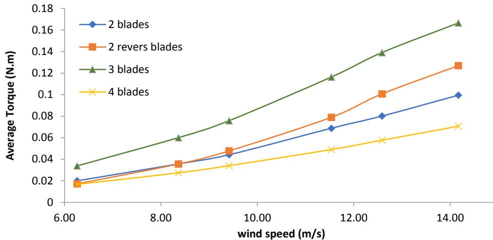
**Figure 15.** Average torque versus wind speed for two, two-reverse, three and four blade IceWind turbines
