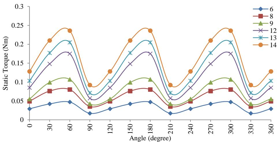
**Figure 18.** Static torque variation with angle of rotation for three blade IceWind turbine.
