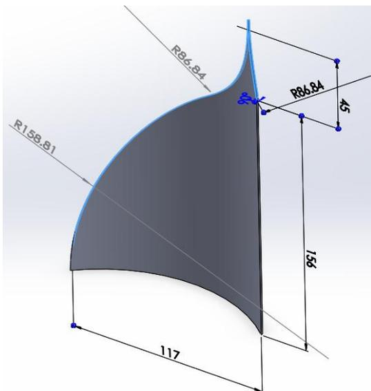
Figure 2. IceWind Blade. Final Design
