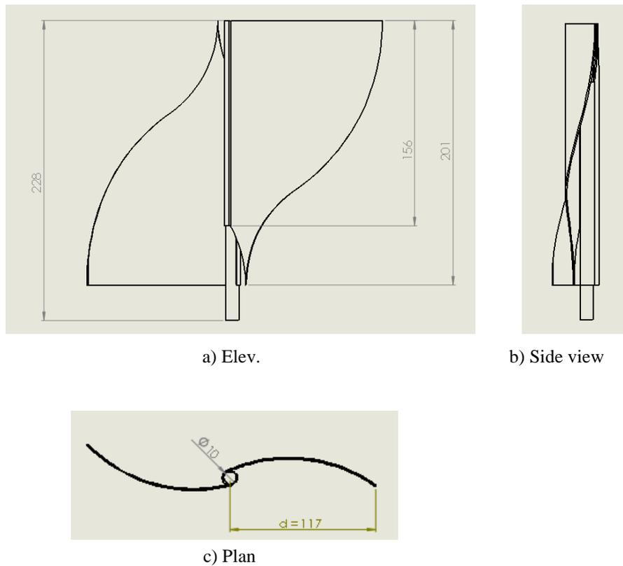
**Figure 8.** Two blade reversed IceWind turbine's three views (Dimensions in mm)
