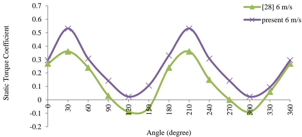
**Figure 24.** Comparison between two blade IceWind and Savonius turbines using static torque coefficient variation with angle of rotation
