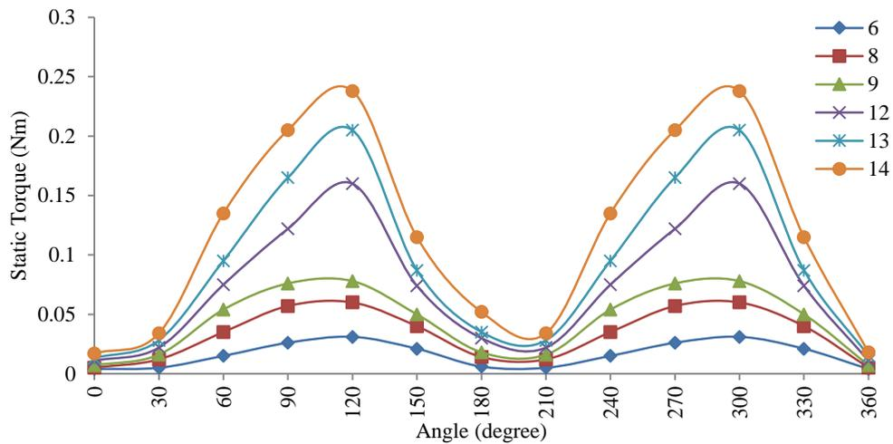
**Figure 17.** Static torque variation with angle of rotation for two-reverse blade IceWind turbine
