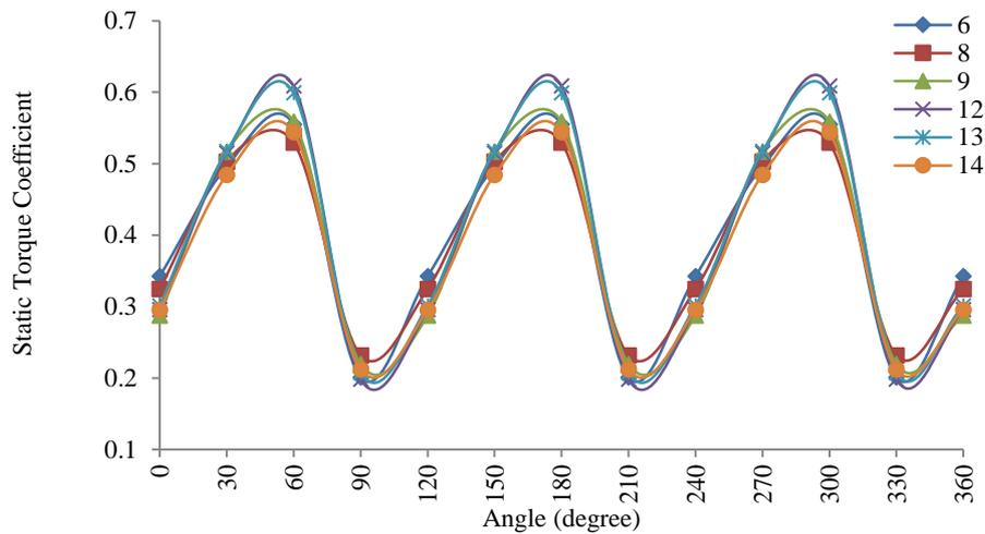
**Figure 22.** Static torque coefficient variation with angle of rotation for three blade IceWind turbine
