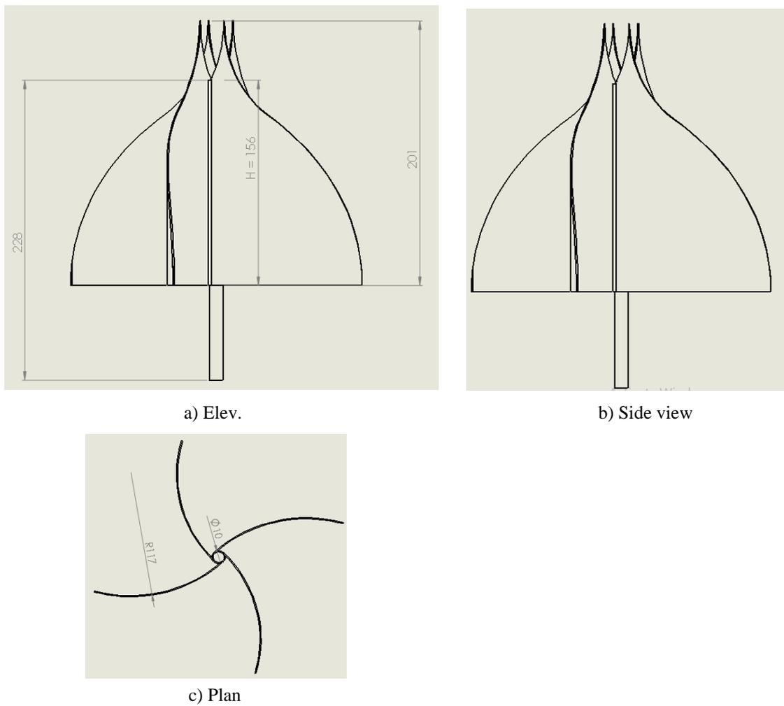
**Figure 12.** Four blade IceWind turbine's three views (Dimensions in mm)
