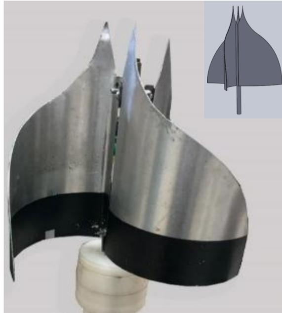
**Figure 9.** A photograph of tested three-blade IceWind turbine
