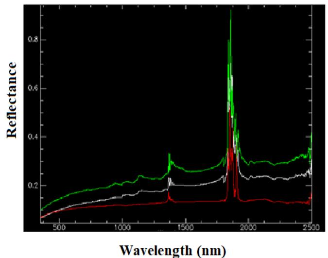
**Figure 3:** Pavement deterioration features spectral library. New pavement (white), Ravelling high severity (green) Ravelling low severity (red)
